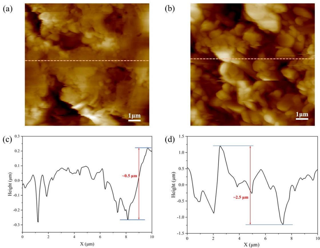
**Figure S9** AFM images of surface morphologies of 1-PVDF before (a) (c) and after irradiation (b) (d).
