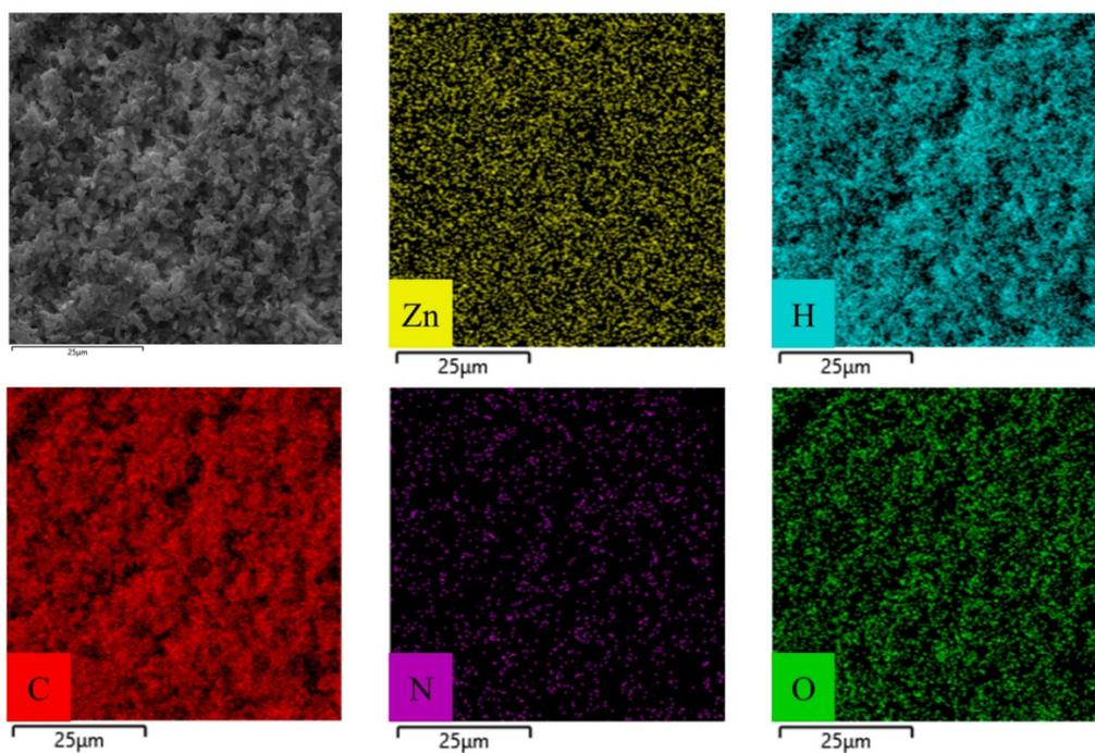
**Figure S7** SEM image and EDS mapping images of the 1-PVDF membrane.
