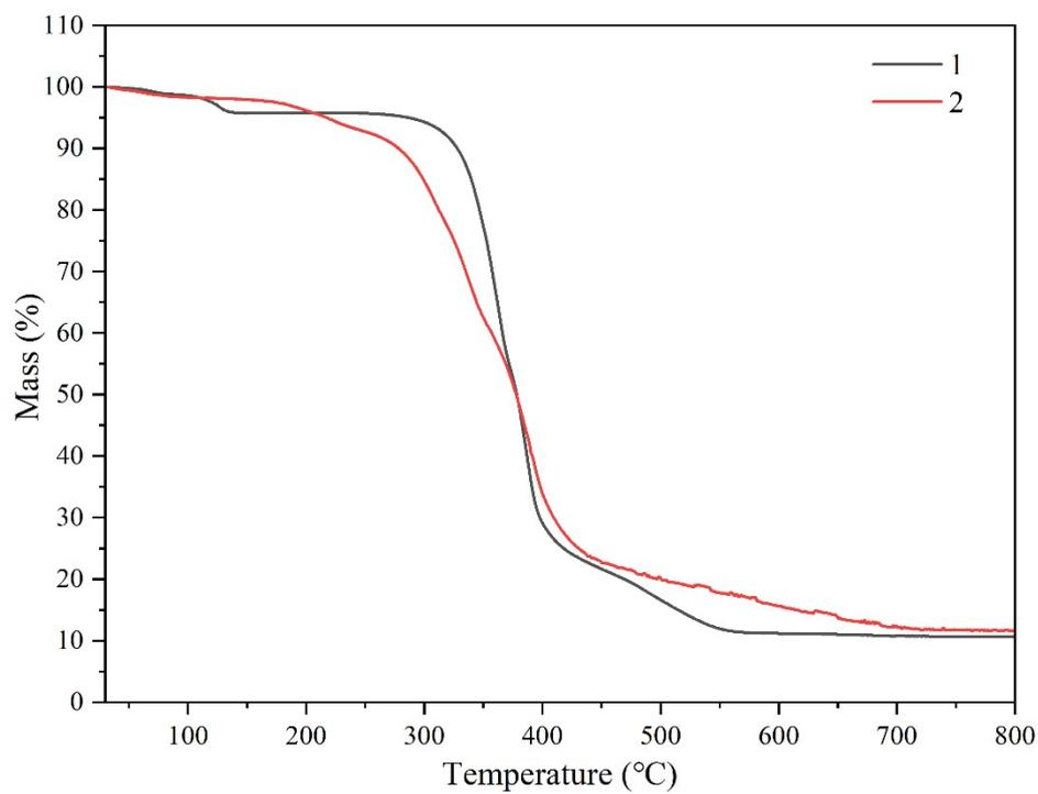
**Fig. S6** TGA plot of **1** and **2** in  $\text{N}_2$  before and after irradiation.
