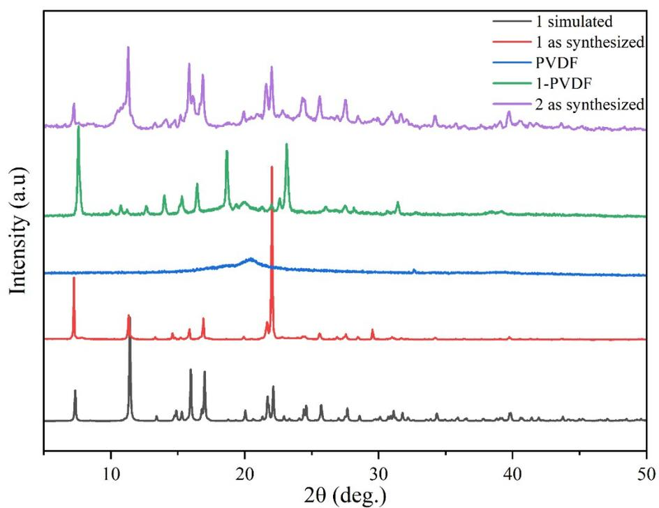
**Figure S2** Powder X-ray diffraction (PXRD) patterns of simulated **1** (black), synthesized **1** (red), **1**-PVDF film (blue), pure PVDF film (green) and synthesized **2** (purple).
