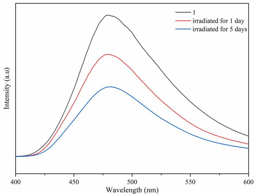
**Figure S5 a)** Fluorescence emission ( $\lambda_{\text{ex}} = 315 \text{ nm}$ ) spectra of **1** before and after irradiation for 1 day and 5 days.
