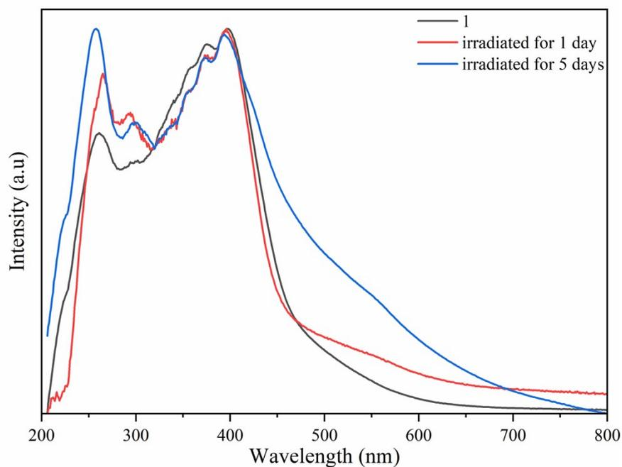
**Figure S1** UV-Vis absorption spectra before and after irradiation for 1 day and 5 days.
