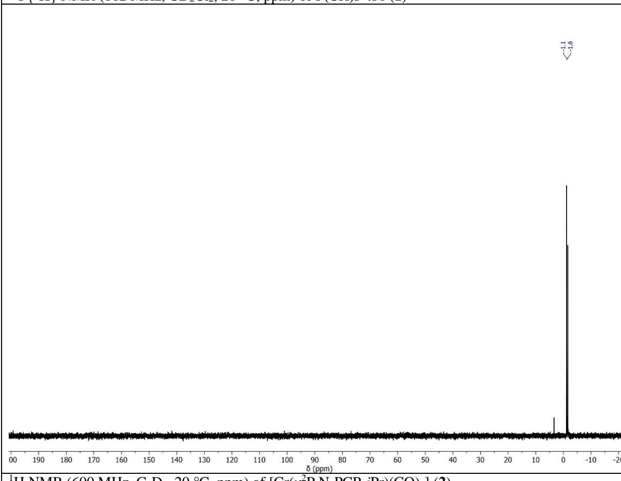
$^1\text{H}$  NMR (600 MHz,  $\text{C}_6\text{D}_6$ , 20 °C, ppm) of  $[\text{Cr}(\kappa^2\text{P},\text{N}-\text{PCP}-i\text{Pr})(\text{CO})_4]$  (**2**)
