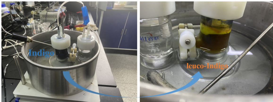
Figure S10. The reaction device for electrocatalytic hydrogenation reduction of indigo
