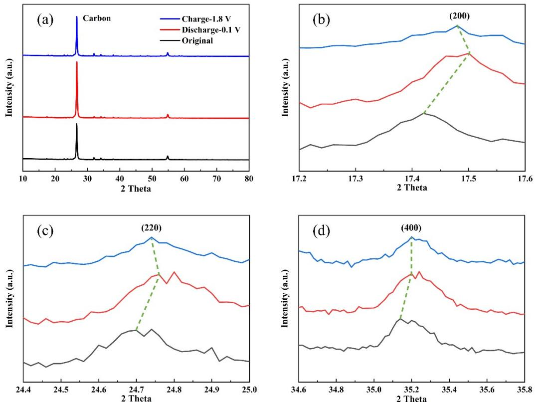
**Fig. S8.** (a) XRD patterns of the FeFe(CN)<sub>6</sub> electrodes under different states after testing in the 0.1 M ZnSO<sub>4</sub>+1 M Na<sub>2</sub>SO<sub>4</sub> electrolyte; (b-d) The magnifications of (200), (220) and (400) peaks.
