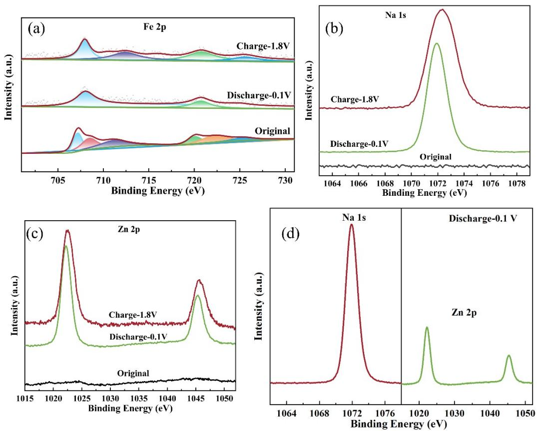
**Fig. S9.** XPS spectra of high resolution Fe 2p (a), Na 1s (b), and Zn 2p (c) in the  $\text{FeFe}(\text{CN})_6$  electrodes at different states; (d) Comparison of Na1s and Zn2p when the  $\text{FeFe}(\text{CN})_6$  electrode is discharged to 0.1V.
