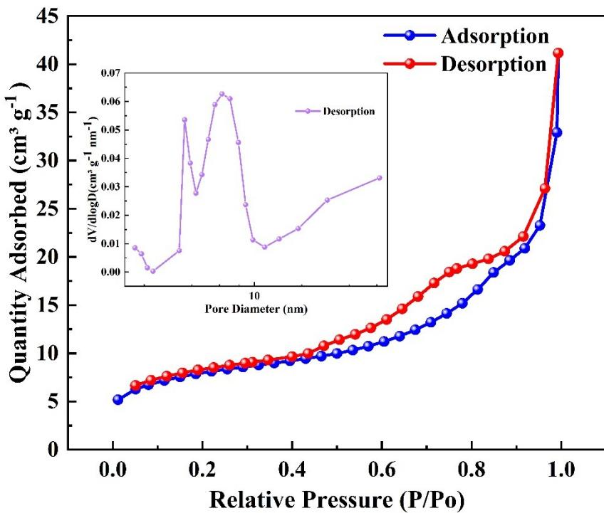
**Fig. S3.**  $\text{N}_2$  adsorption-desorption isotherm and pore-size distribution curve of  $\text{FeFe}(\text{CN})_6$ .
