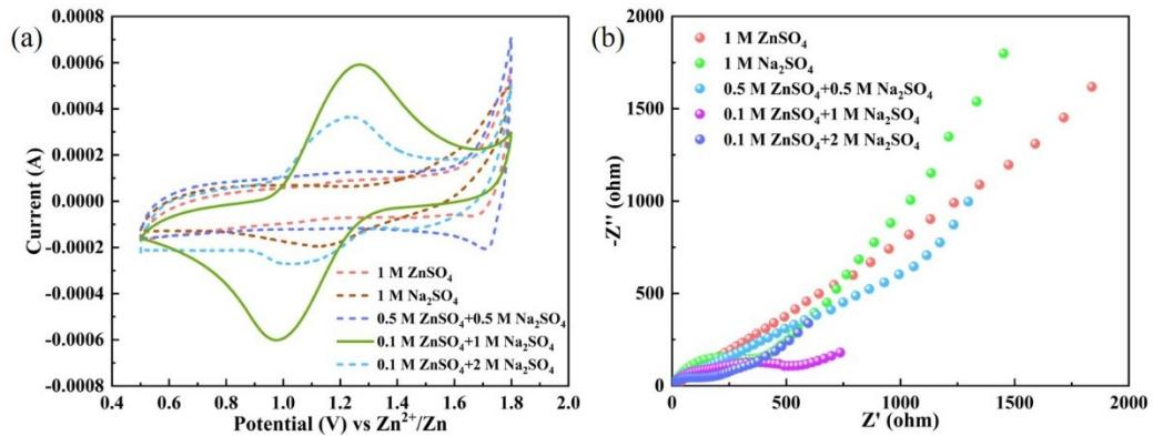
**Fig. S4.** (a) CV and (b) EIS curves of  $\text{FeFe}(\text{CN})_6$  after 200 cycles in different electrolytes.
