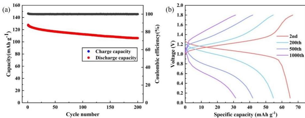
**Fig. S6.** Electrochemical performances of Zn//FeFe(CN)<sub>6</sub> cells in 0.1 M ZnSO<sub>4</sub>+1 M Na<sub>2</sub>SO<sub>4</sub> electrolyte. (a) Cycling performance at 15C for 200 cycles; (b) GCD curves in different cycles at 20C.
