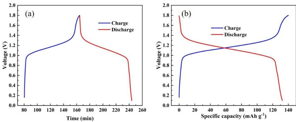
**Fig. S7.** Charge-discharge curves of Zn//FeFe(CN)<sub>6</sub> cells in 0.1 M ZnSO<sub>4</sub>+1 M Na<sub>2</sub>SO<sub>4</sub> electrolyte.
