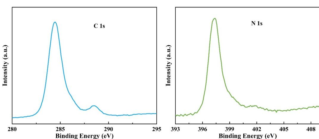
**Fig. S10.** XPS spectra of high resolution C 1s and N 1s in the  $\text{FeFe}(\text{CN})_6$  electrodes.
