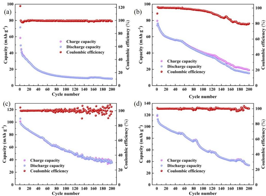
**Fig. S5.** Cycling performance of Zn//FeFe(CN)<sub>6</sub> battery at 1C in different electrolytes: (a) 1 M ZnSO<sub>4</sub> electrolyte; (b) 1 M Na<sub>2</sub>SO<sub>4</sub> electrolyte; (c) 0.5 M ZnSO<sub>4</sub>+0.5 M Na<sub>2</sub>SO<sub>4</sub> electrolyte; (d) 0.1 M ZnSO<sub>4</sub>+2 M Na<sub>2</sub>SO<sub>4</sub> electrolyte.
