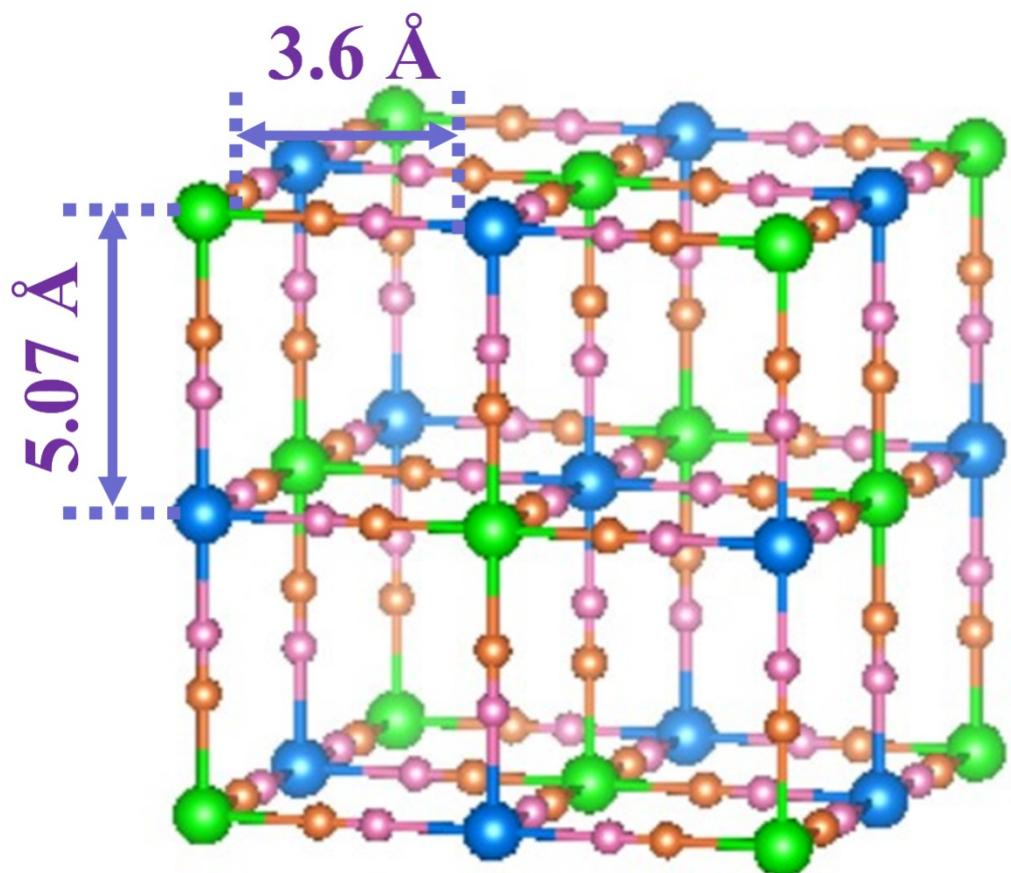
**Fig. S1.** The structure of  $\text{FeFe}(\text{CN})_6$ .
