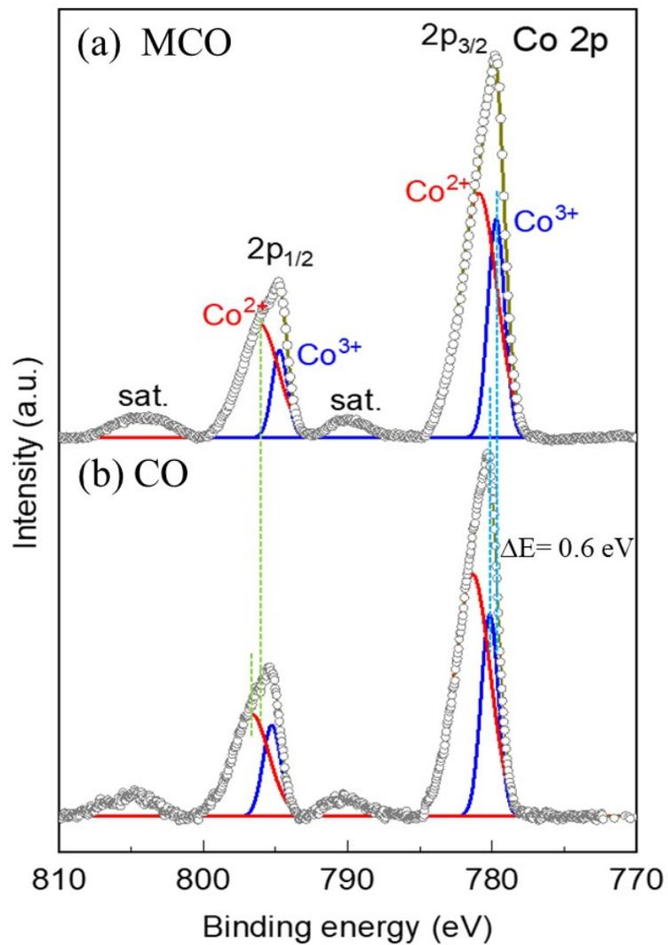
**Figure S4.** High-resolution Co 2p XPS spectra of (a) MCO, and (b) CO.
