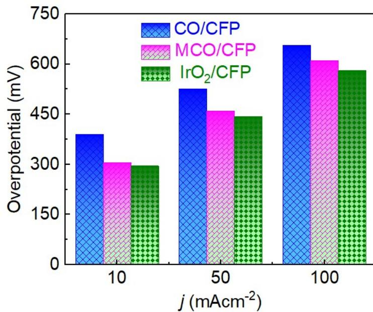
Figure S5. OER overpotential vs current density profile.
