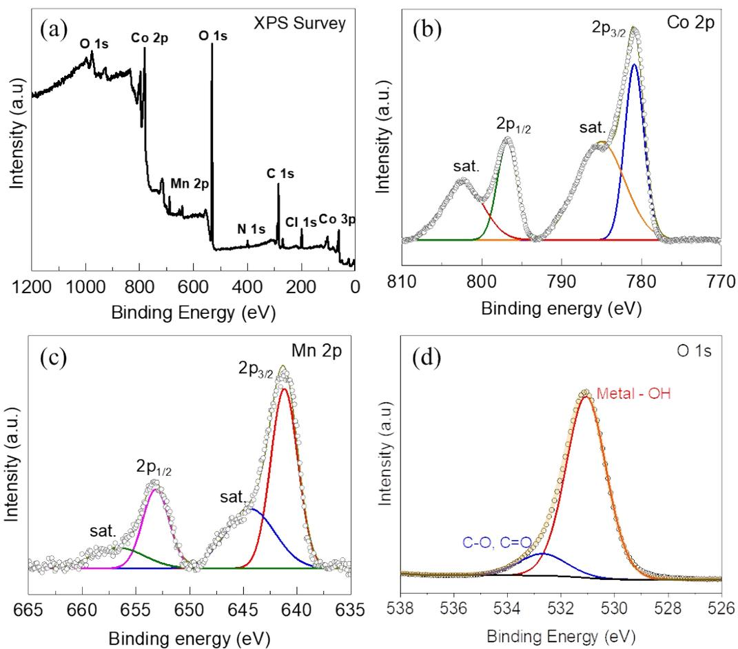
**Figure S3.** (a) XPS survey spectrum of the MCHC film, the corresponding high-resolution XPS spectrum of (b) Co 2p, (c) Mn 2p, and (d) O 1s.
