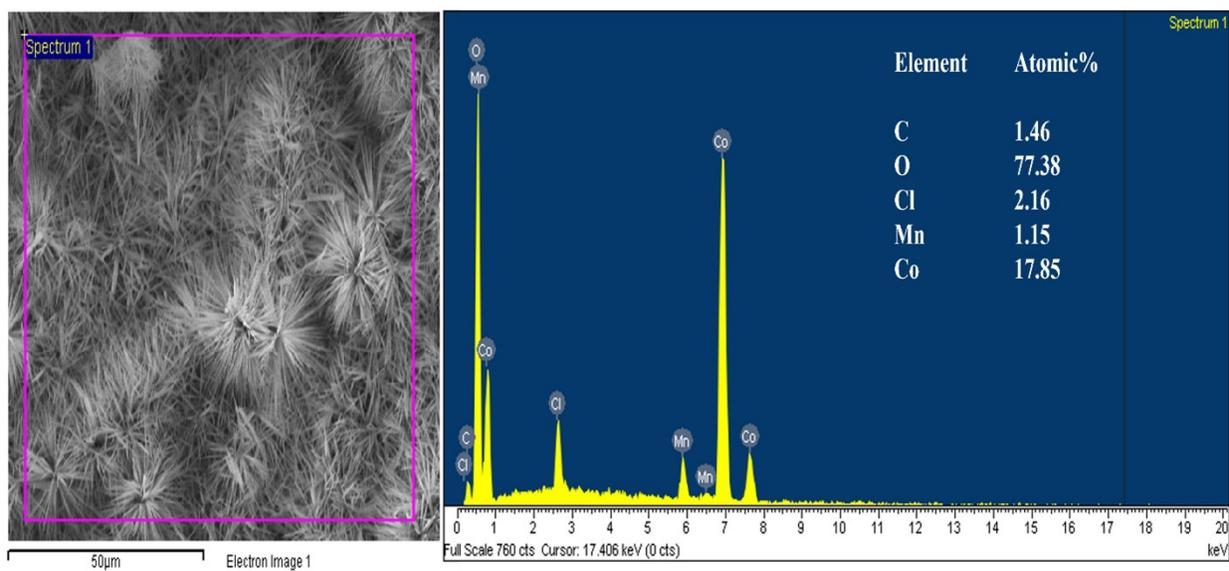
**Figure S2.** EDX spectrum of the MCHC film.
