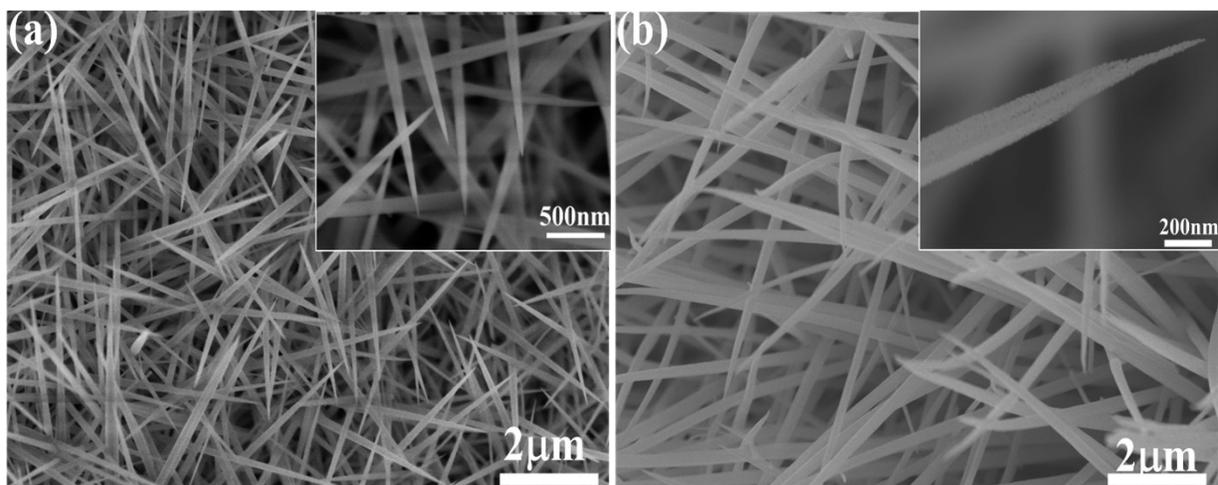
**Figure S1.** SEM images of (a) cobalt hydroxycarbonate (CHC) film and (b)  $\text{Co}_3\text{O}_4$  (CO) film.
