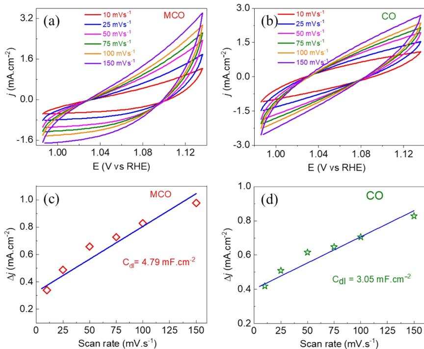
**Figure S6.** (a)-(b) Cyclic voltammograms of various electrodes in 1.0 M KOH aqueous electrolyte at different potential scanning rates ( $\text{m.Vs}^{-1}$ ); (c)-(d) Linear plots obtained by plotting the average current density ( $\Delta j$ ) vs potential scanning rates at 1.061V vs RHE .
