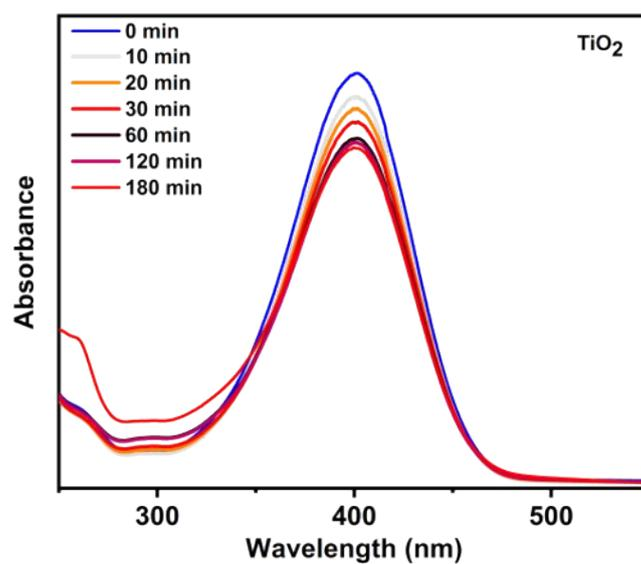
**Figure S6.** The absorbance spectra during the reduction process of 4-nitrophenol using TiO<sub>2</sub> as catalyst.
