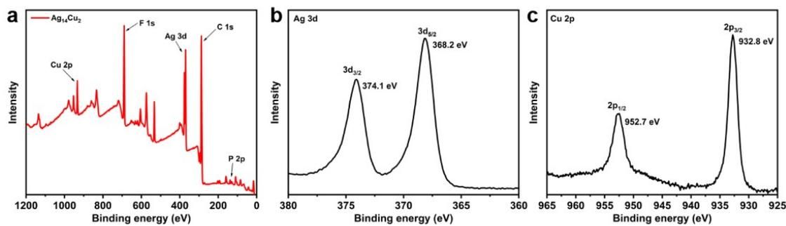
**Figure S4.** (a) XPS survey-scan spectra of the  $\text{Ag}_{14}\text{Cu}_2$  nanoclusters; High-resolution (b) Ag 3d and (c) Cu 2p XPS spectrum of the  $\text{Ag}_{14}\text{Cu}_2$  nanoclusters.
