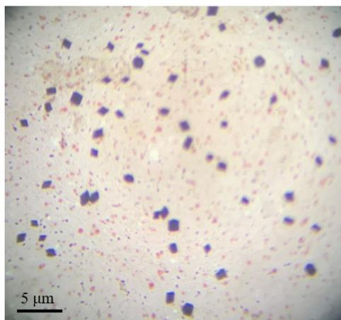
**Figure S1.** The images of  $\text{Ag}_{14}\text{Cu}_2$  crystals under an optical microscope.
