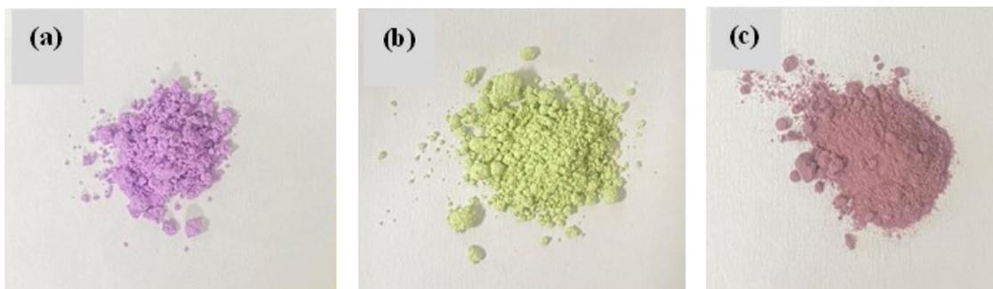
**The obtained (a) CoMoS<sub>4</sub>, (b) NiMoS<sub>4</sub>, and (c) CoNiMoS<sub>4</sub> particles via hydrothermal technique**
