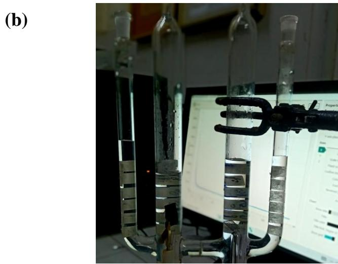
**Fig. S11** (a) Faradic efficiency of **[1a]ClO<sub>4</sub>** and (b) demonstration of the two compartment H-cell used for the Faradaic efficiency determination.
