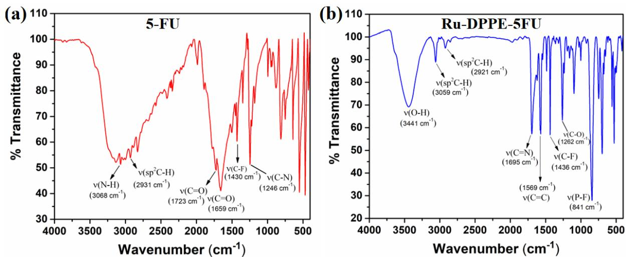
**Fig. S1.** The solid-state FT-IR spectrum of **5-FU** (a), and  $[\text{Ru}(\text{dppe})_2(5\text{-FU})]\text{PF}_6$  (**Ru-DPPE-5FU**) (b) in KBr.
