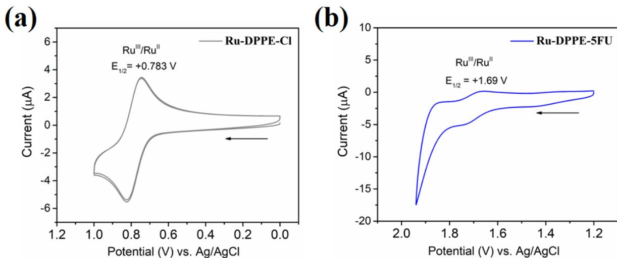
**Fig. S9.** Cyclic Voltammograms of (a) **Ru-DPPE-Cl** and (b) **Ru-DPPE-5FU** in dichloromethane (0.1M TBAPF<sub>6</sub>) at 100 mV/sec scan rate.
