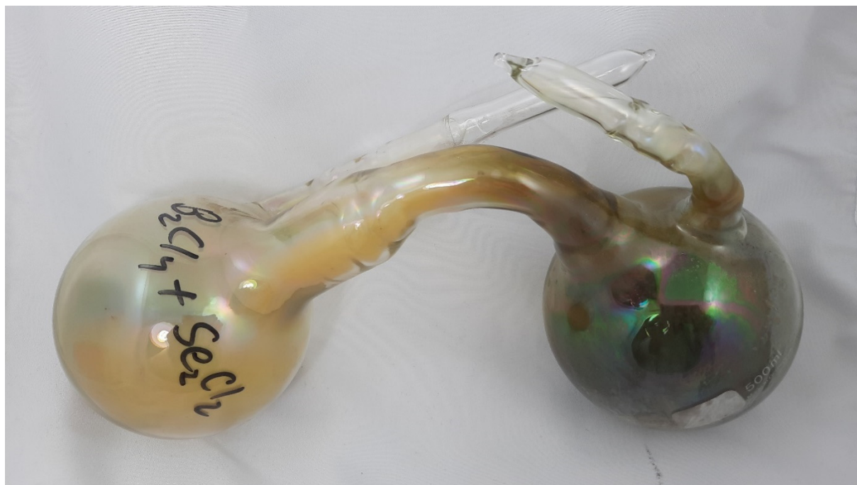
Fig. S12: Sealed pyrolysis double-flask after reaction before work-up.
