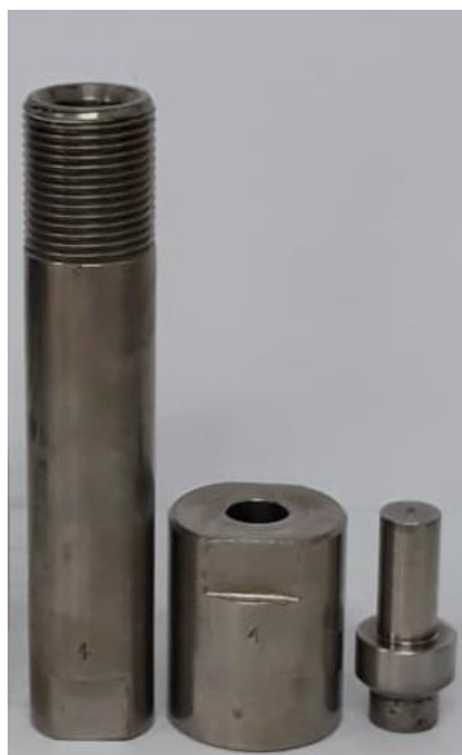
Figure S28. Stainless steel reactor used in syntheses of compounds 1-3 .
