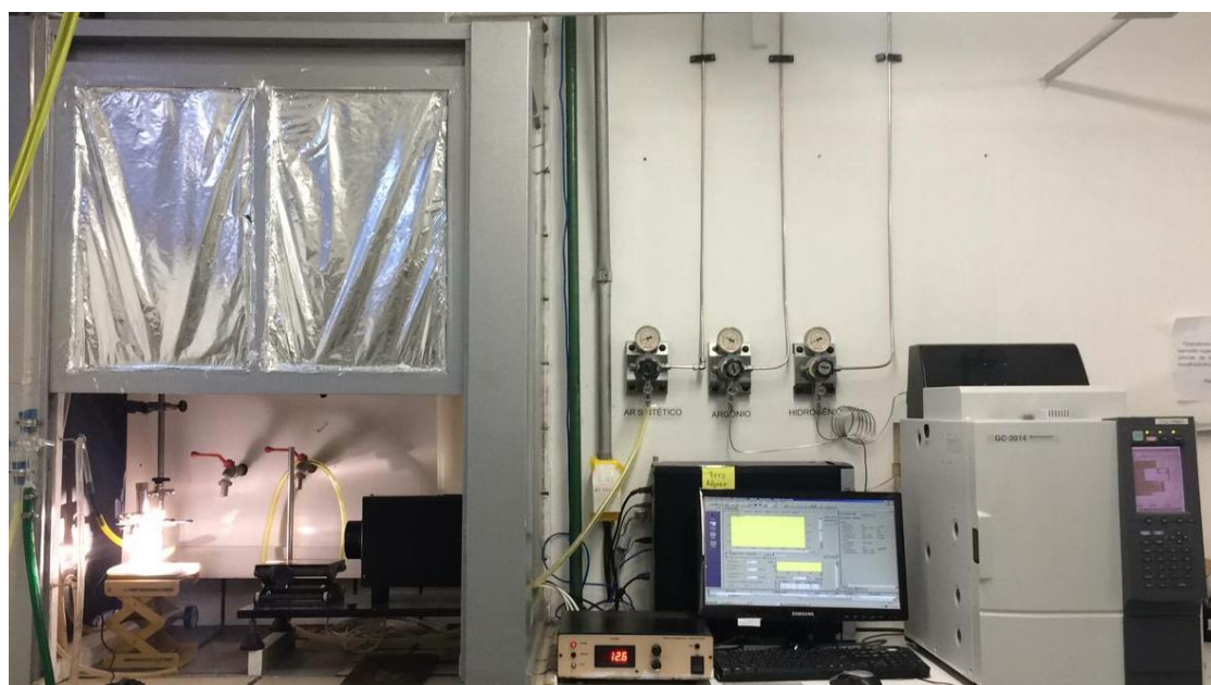
Figure S29. System used in experiments applying photocatalyst TiO 2 -1A and TiO 2 -2A for hydrogen evaluation.
