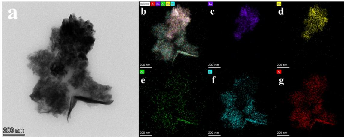
**Fig. S3** TEM image of (a)  $\text{CoSe}_2@ZnIn_2S_4$  physical mixture heterostructure and (b) the corresponding EDS and elemental mapping images of (c) Co, (d) Se, (e) Zn, (f) In, and (g) S.
