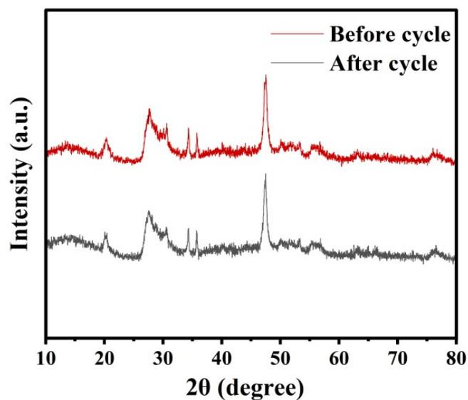
**Fig. S5** XRD patterns comparison of  $\text{CoSe}_2/\text{ZnIn}_2\text{S}_4$ -20 before and after cycle.
