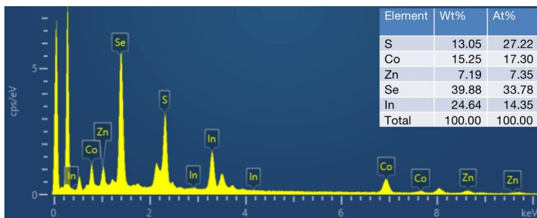
**Fig. S2** EDS element analysis of CoSe<sub>2</sub>/ZnIn<sub>2</sub>S<sub>4</sub>-20.
