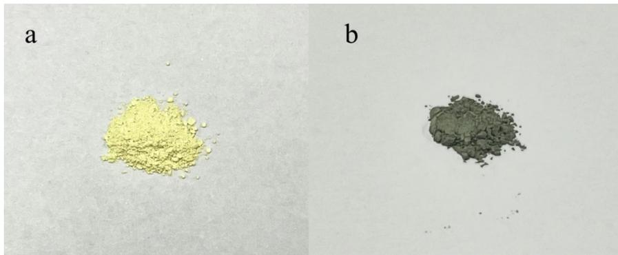
**Fig. S4** the pictures of (a)  $ZnIn_2S_4$  and (b)  $\text{CoSe}_2/ZnIn_2S_4-20$  sample.
