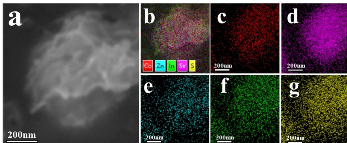
**Fig. S1** SEM image of (a) CoSe<sub>2</sub>/ZnIn<sub>2</sub>S<sub>4</sub>-20 core-shell heterostructure and (b) the corresponding EDS and elemental mapping images of (c) Co, (d) Se, (e) Zn, (f) In, and (g) S.
