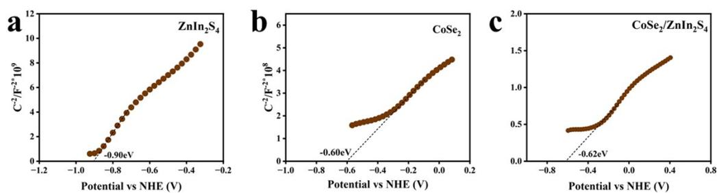
**Fig. S6** Mott-Schottky plots of (a)  $\text{ZnIn}_2\text{S}_4$ , (b)  $\text{CoSe}_2$  and (c)  $\text{CoSe}_2/\text{ZnIn}_2\text{S}_4$ -20.
