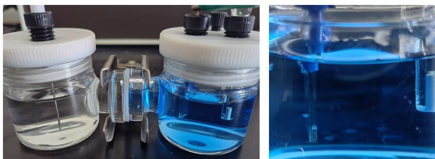
Fig. S38 The photograph of the H-shape electrolyte cell and the oxygen generated on the surface of ITO electrode during the CPE test of complex 1 .
