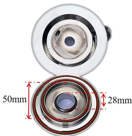
Figure S1. Physical diagram and size of the reaction chamber.
