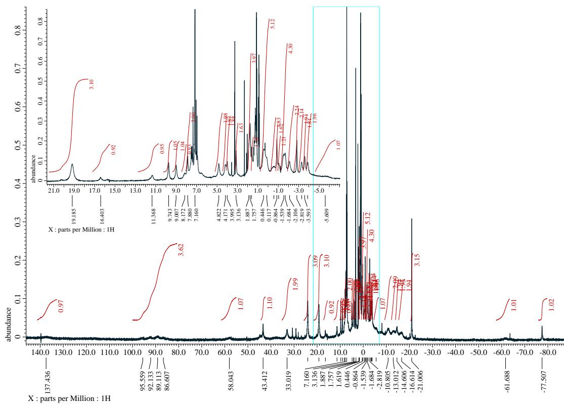
**Figure S3.**  $^1\text{H}$  NMR spectrum of **2** in  $\text{C}_6\text{D}_6$  at room temperature.
