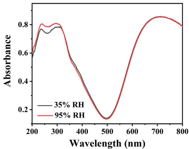
**Fig. S13** UV-Vis DRS of CH<sub>3</sub>-Cu(BDC) after exposed to different relative humidity.
