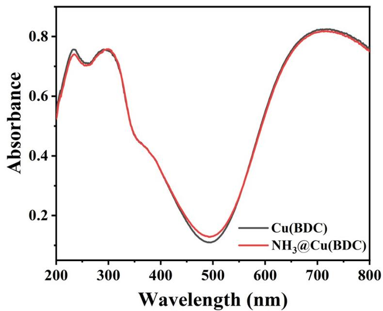
**Fig. S9** UV-vis DRS of Cu(BDC) exposed to 50 ppm NH<sub>3</sub> for 25 min.
