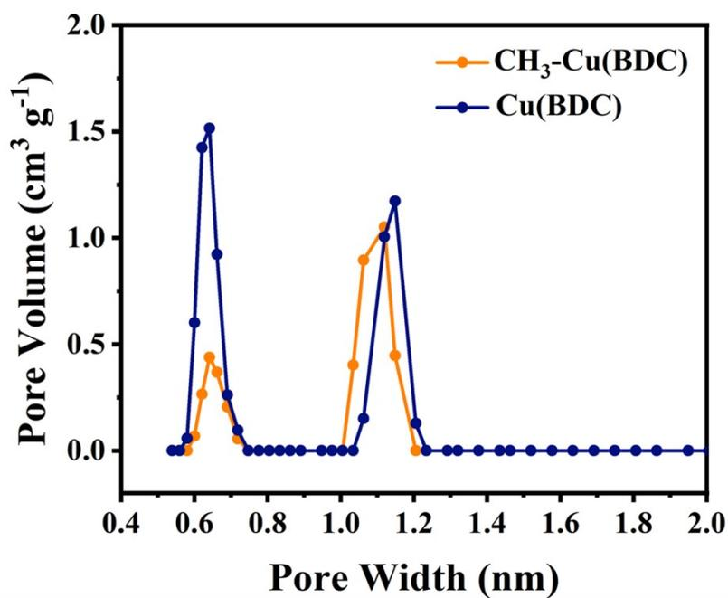
**Fig. S6** The pore-size distribution of  $CH_3-Cu(BDC)$  and  $Cu(BDC)$ .
