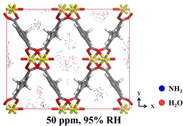
**Fig. S18** GCMC simulations of the competitive adsorption between  $\text{H}_2\text{O}$  and  $\text{NH}_3$  on  $\text{CH}_3\text{-Cu}(\text{BDC})$  (50 ppm  $\text{NH}_3$ , 95 % RH).
