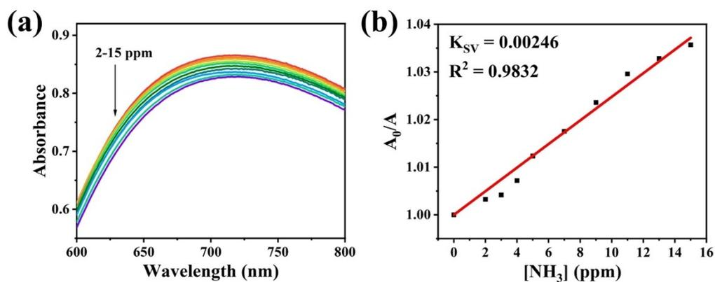
**Fig. S11** (a) UV-Vis DRS of CH<sub>3</sub>-Cu(BDC) after exposed to 2, 3, 4, 5, 7, 9, 11, 13 and 15 ppm ammonia. (b) Absorbance curve over ammonia levels.
