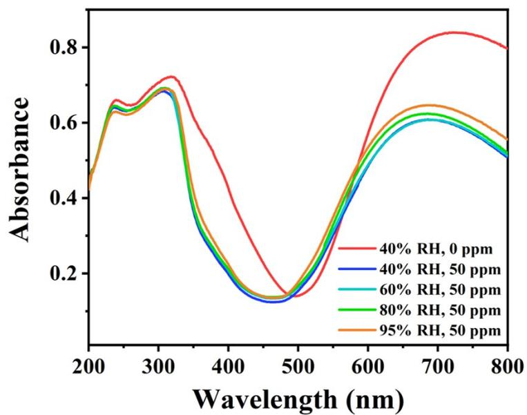
**Fig. S14** UV-Vis DRS of CH<sub>3</sub>-Cu(BDC) exposed to 50 ppm NH<sub>3</sub> with different relative humidity.
