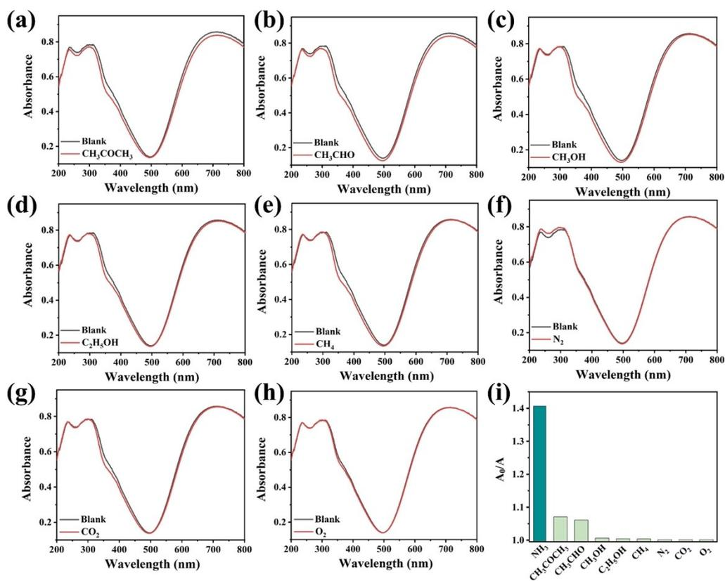
**Fig. S15** Response of CH<sub>3</sub>-Cu(BDC) against NH<sub>3</sub> and other exhaled air. The concentration of acetone, acetaldehyde, methanol and ethanol were 50 ppm, the rest of gases were high-purity.
