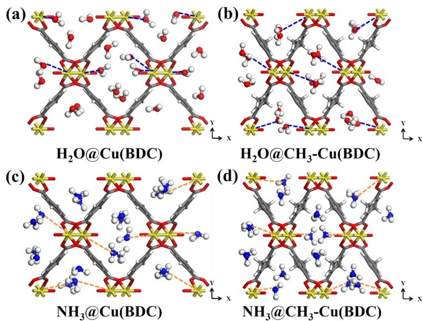
**Fig. S17** GCMC simulations of  $\text{H}_2\text{O}$  and  $\text{NH}_3$  adsorption sites in  $\text{Cu}(\text{BDC})$  and  $\text{CH}_3\text{-Cu}(\text{BDC})$ .
