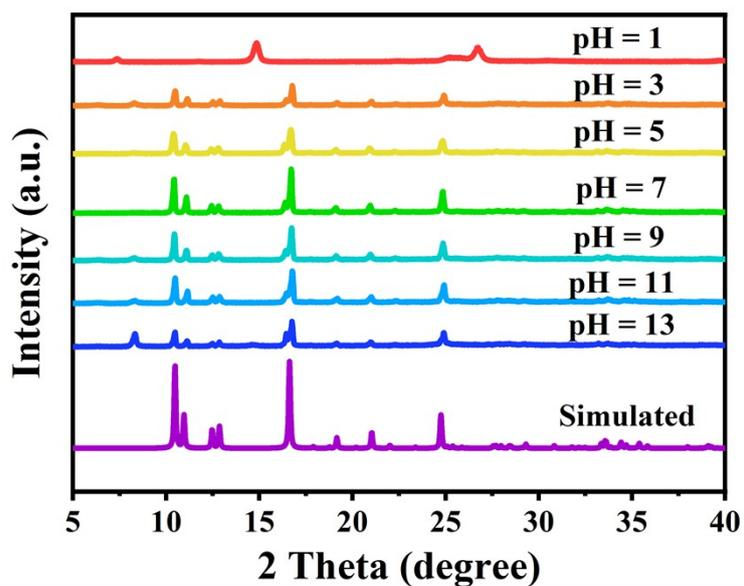
**Fig. S4** PXRD profiles of CH<sub>3</sub>-Cu(BDC) samples soaked in the aqueous solutions with pH = 1, 3, 5, 7, 9, 11, 13 solution for 24 h.
