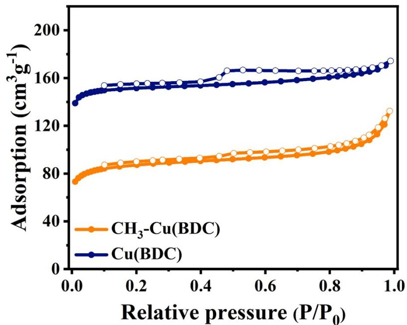
**Fig. S5**  $N_2$  sorption isotherms of  $CH_3-Cu(BDC)$  and  $Cu(BDC)$  at 77 K. The Brunauer-Emmett-Teller (BET) surface area was  $339\text{ m}^2\text{g}^{-1}$ , there is decreased by 44% compared with  $Cu(BDC)$  ( $603\text{ m}^2\text{g}^{-1}$ )
