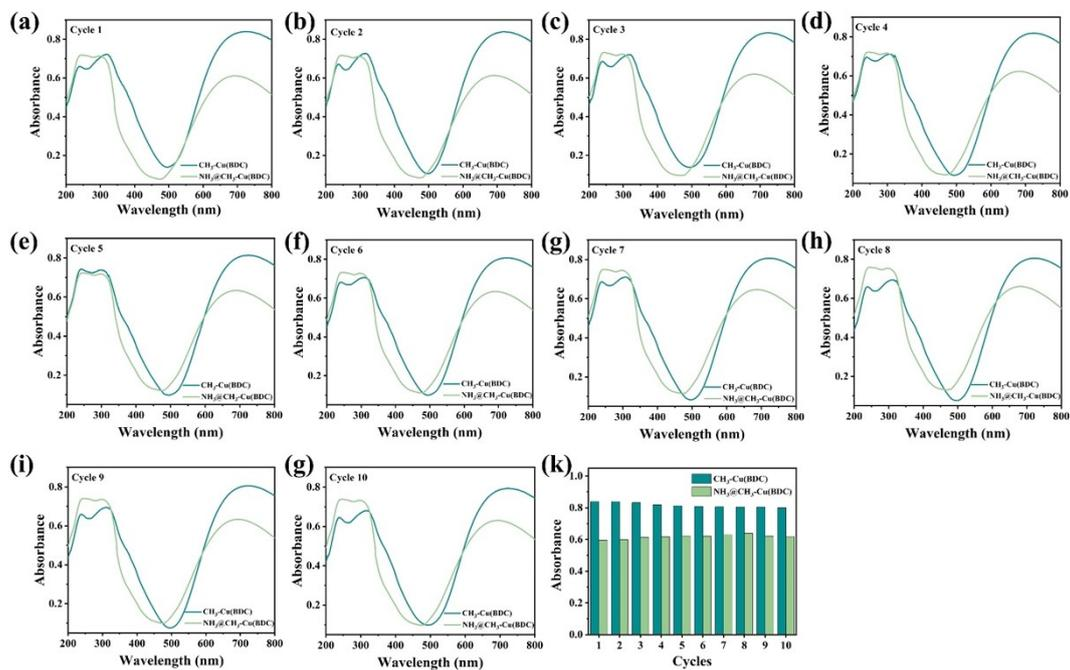
**Fig. S23** Response to  $\text{NH}_3$  (50 ppm) during 10 cycles of adsorption and desorption.
