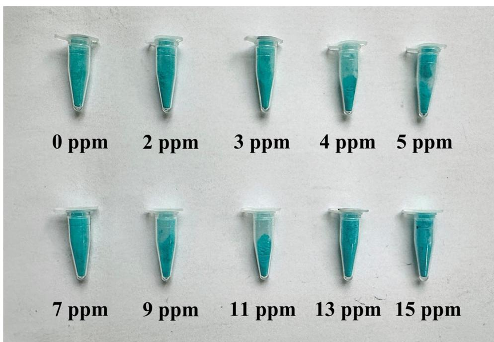
**Fig. S12** Digital images of CH<sub>3</sub>-Cu(BDC) after exposed to 2, 3, 4, 5, 7, 9, 11, 13 and 15 ppm ammonia.
