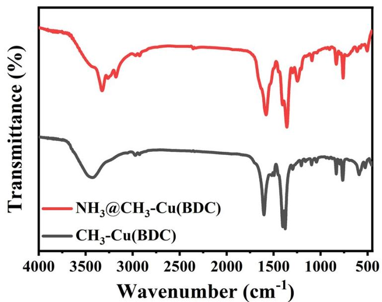
**Fig. S10** FT-IR spectra of CH<sub>3</sub>-Cu(BDC) and NH<sub>3</sub>@CH<sub>3</sub>-Cu(BDC).
