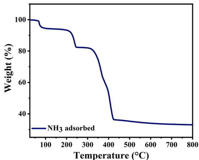
**Fig. S22** TGA curves of  $\text{NH}_3@CH_3\text{-Cu(BDC)}$  under  $\text{N}_2$  flow. The result show that the  $\text{NH}_3$  in  $\text{NH}_3@CH_3\text{-Cu(BDC)}$  will be desorbed at 80 °C
