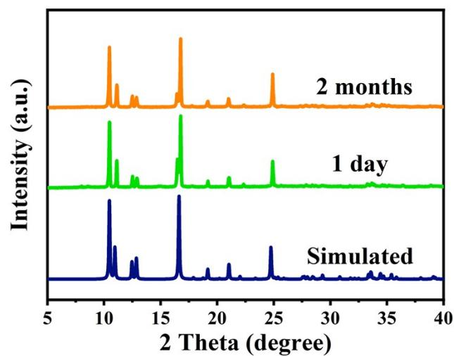
**Fig. S20** PXR D patterns of CH<sub>3</sub>-Cu-BTC for 1 day and 2 months in the atmospheric environment.
