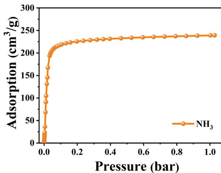
Fig. S7 Ammonia adsorption isotherm of CH<sub>3</sub>-Cu(BDC).
