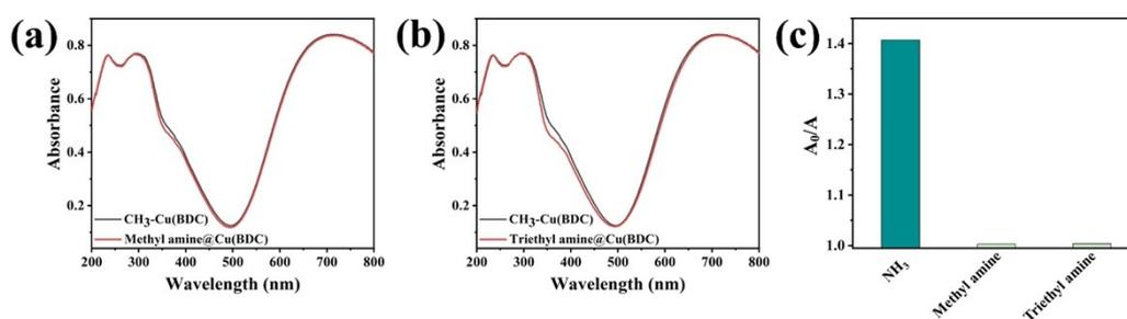
**Fig. S16** (a-b) UV-Vis DRS of CH<sub>3</sub>-Cu(BDC) exposed to 50 ppm methyl amine (a) and triethyl amine (b) atmosphere. (c) Response of CH<sub>3</sub>-Cu(BDC) against NH<sub>3</sub> and bulkier amines.
