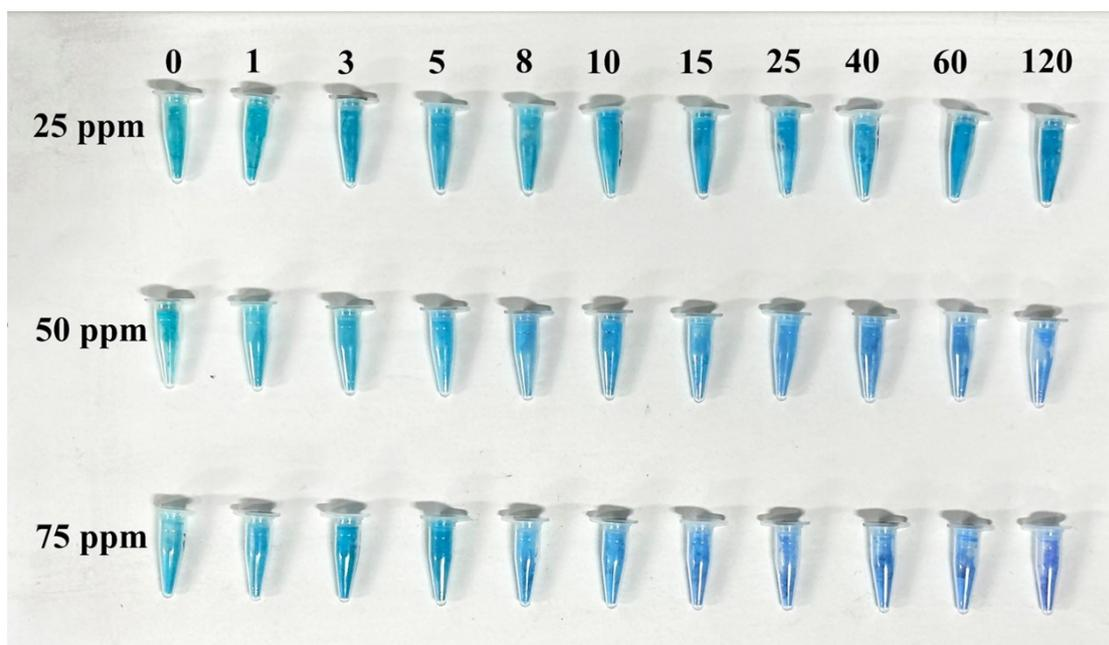
Fig. S8 Digital images of CH<sub>3</sub>-Cu(BDC) after exposed to 25, 50 and 75 ppm NH<sub>3</sub> for different times.
