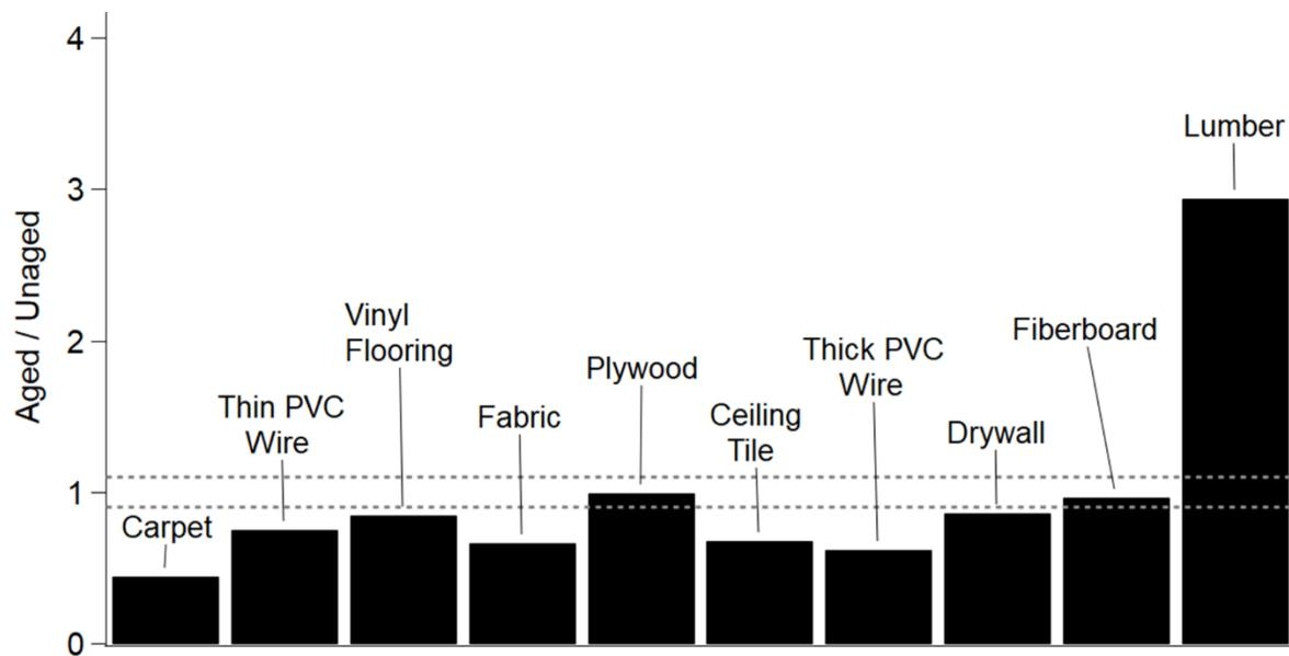
**Figure S12.** Ratios of the 2 h aged to unaged integrated, UV range *MAC* values. The reported ratios were calculated by integrating the *MAC* values in the UV range (280-400 nm) then referencing the 2 h aged integrated *MAC* value to that of the unaged, integrated *MAC* value. The dashed line (0.9 to 1.1) indicates the threshold for the change.
