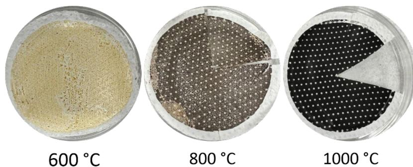
**Figure S2.** Sample photographs of filters containing OA generated through the pyrolysis of carpet at 600, 800, and 1000 °C under N<sub>2</sub>. Pyrolysis temperatures greater than 600 °C yielded OA that was poorly soluble due to presence of black carbon (BC).
