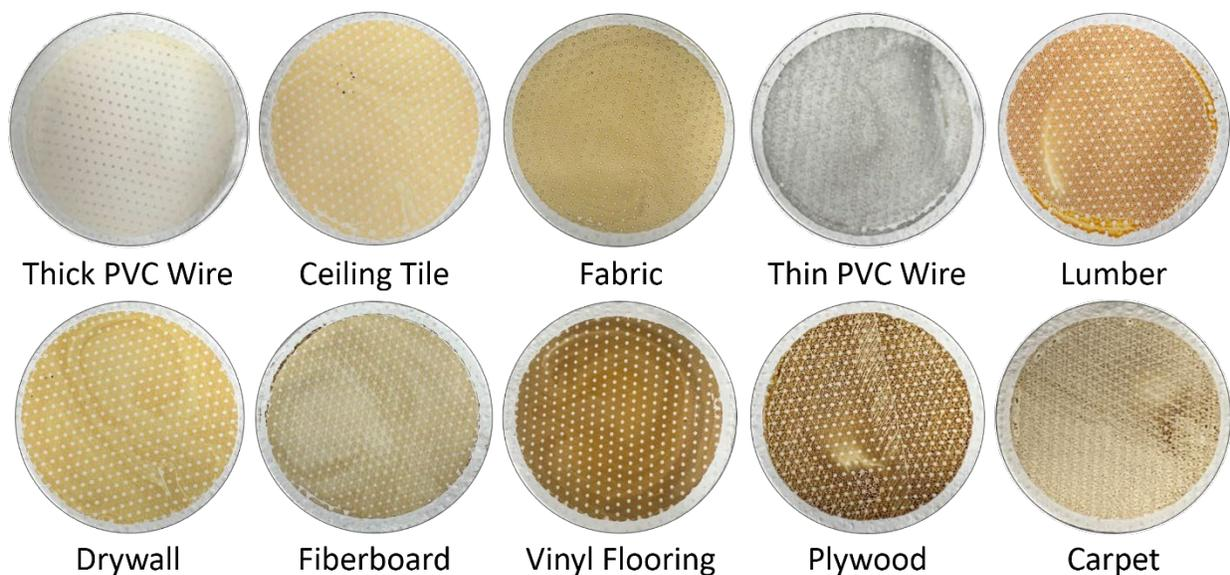
**Figure S1.** Sample photographs of filters containing organic aerosol (OA) generated through the pyrolysis of ten urban materials at 600 °C under N<sub>2</sub>. The OA differed in appearance amongst urban materials.
