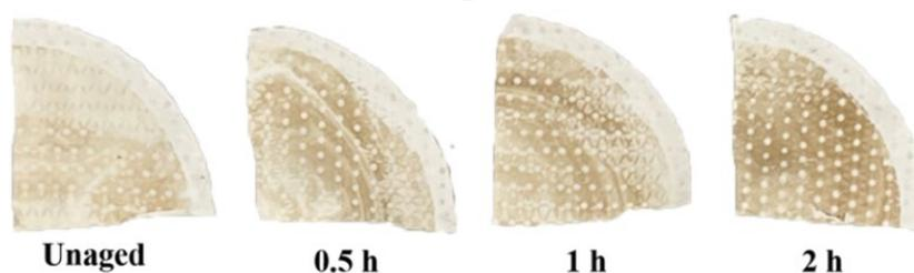
**Figure S8.** Pictures of Teflon filters after photolysis and subsequent extraction of lumber OA (a), fabric OA (b), and vinyl tile OA (c). Orgmix was used in the extraction of all OA. Only these 3 urban materials left behind residual OA on Teflon filters after extraction.
