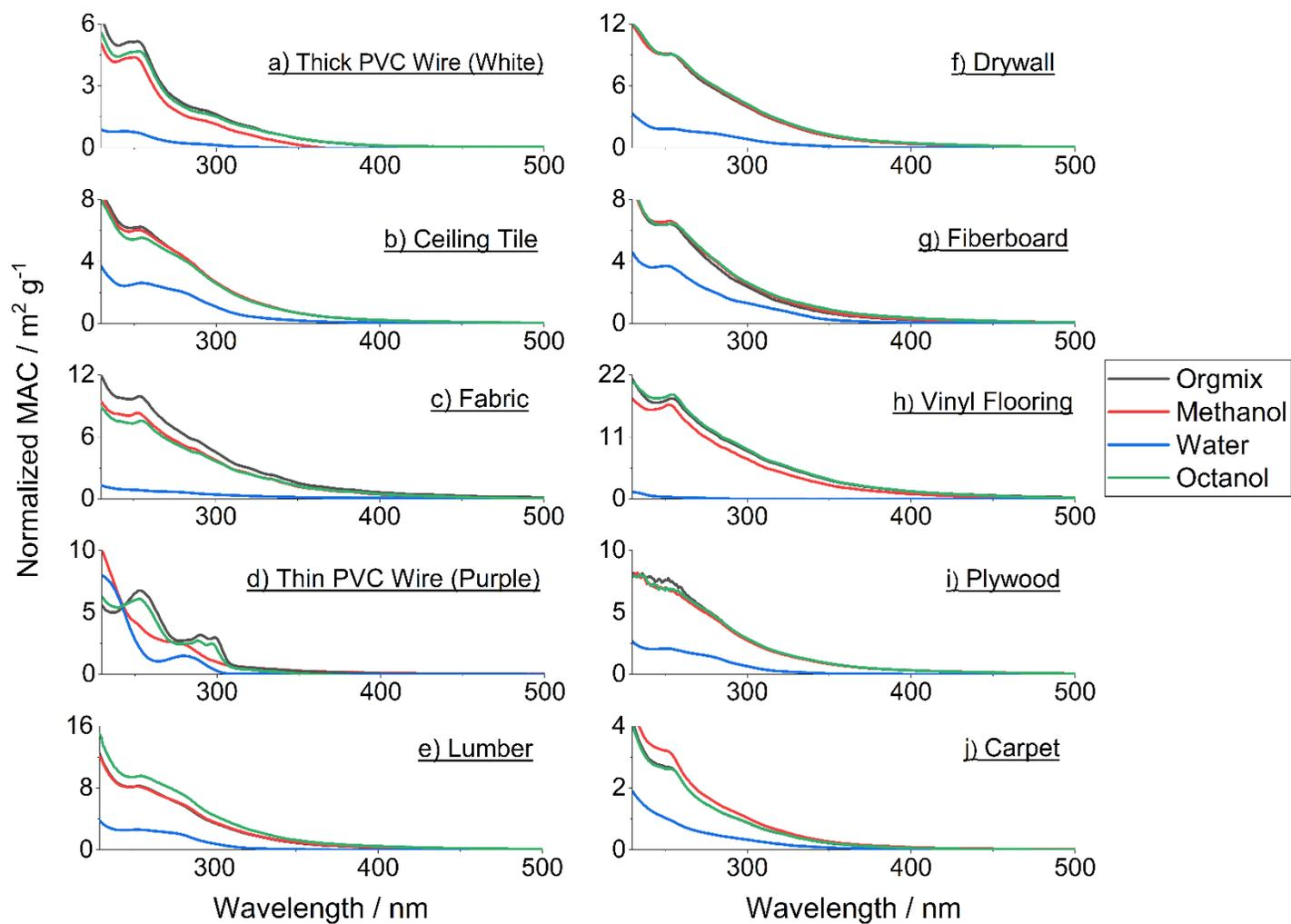
**Figure S3.** UV-Vis absorption spectra recorded after the pyrolysis of urban materials (a-j) and extraction in orgmix (grey), methanol (red), water (blue), and n-octanol (green). The *MAC* values assume complete extraction of OA from the filter. The lowest *MAC* observed for water indicates that it does not extract the OA fully and is the least effective solvent tested for all materials. Plywood extracts were diluted by a factor of ten for absorbance measurements.
