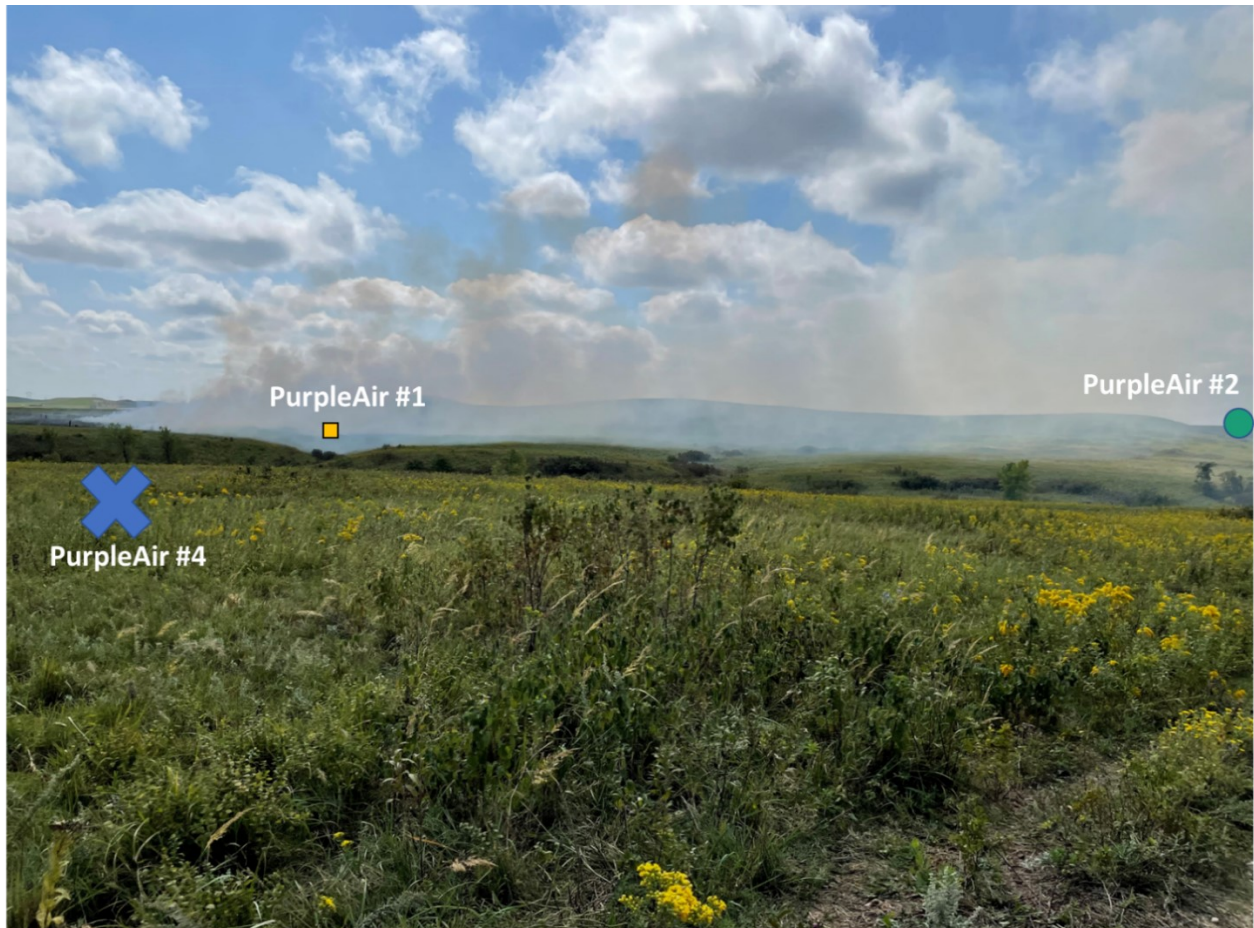
352 Figure S15: Image of plume from near upwind (PurpleAir #4) location. The downwind – close (PurpleAir #1) and 353 downwind – mid (PurpleAir #2) locations are also indicated. An example of the wind conditions causing the plume to 354 fumigate the valley.
