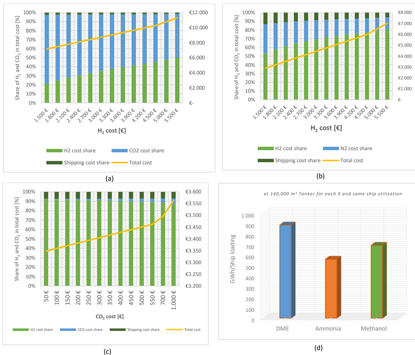
Figure S2: a,b and c) Evaluations at shipping distance of 20,000 km (a) Cost structure of MeOH production at CO 2 cost from DAC. (b) Cost structure of NH 3 production at N 2 cost from ASU (c) The cost structure for delivery of 1 ton of H 2 at the utilization point using DME as H 2 carrier in a closed DME/CO 2 cycle as a function of CO 2 cost. (d) a comparison of the energy delivered if the same ship capacity is considered for all the three carriers.
