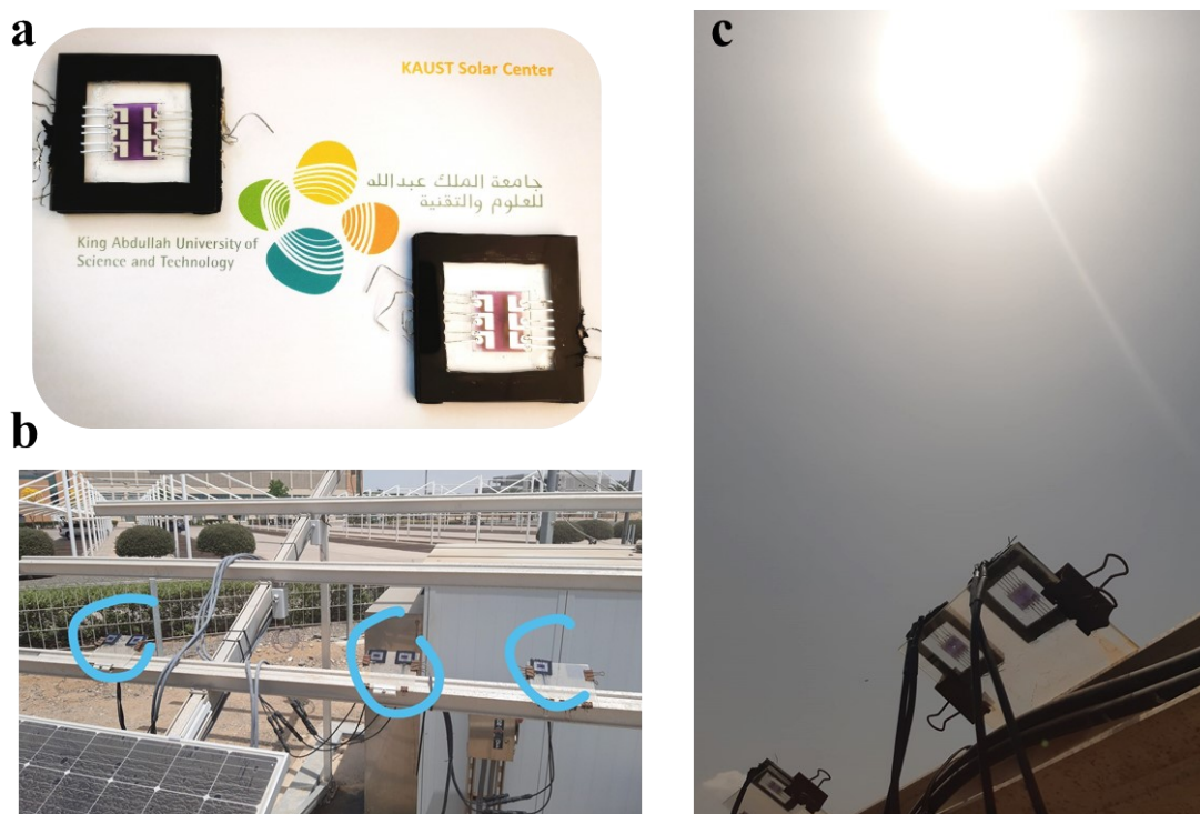
Figure S22. a The encapsulated D18-based terpolymer devices for outdoor stability test. b-c The photos of the outdoor stability test site in KAUST campus.
