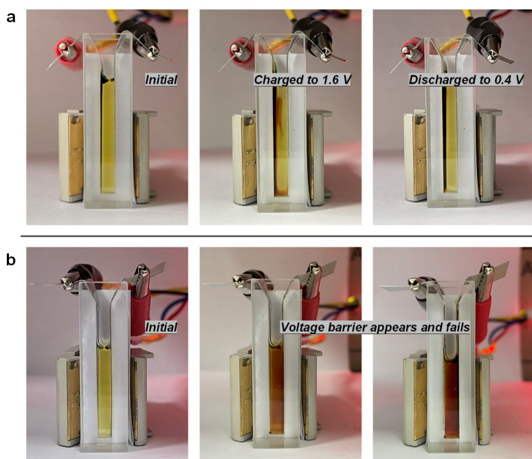
Figure S30. Optical images in the different states of Zn/NVO-PAC cuvette cells with (a) 3-01-90 and (b) 3-01-00, respectively.
