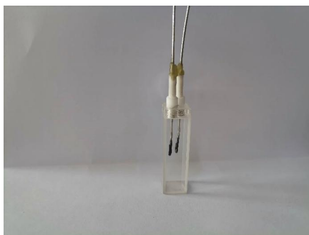
Fig. S23 Schematic diagram of electrolytic cell (Na || Na) device for in situ optical microscopy.
