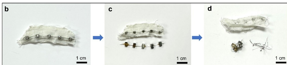
Fig. S17. Recycle process of \text{Bi}_2\text{Te}_3 based TET. (a) A diagram of recycle process of TET, (b-d) Physical disassembling process of TET: (b) A small unit of TET, (c) Heating the weld and disassemble the TE pillars, (d) Removing the tin-plated copper wires from fabric.
