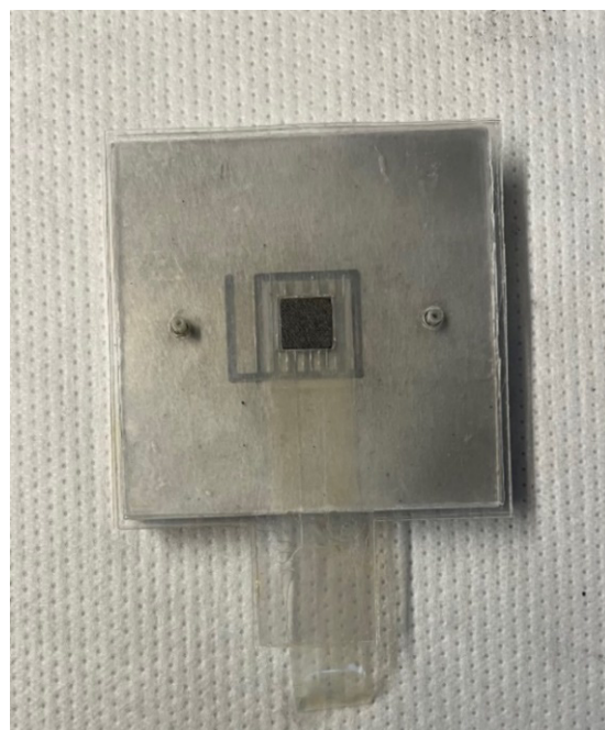
Figure S10. Cathode PTE placed on top of the AEM, completing the MEA.
