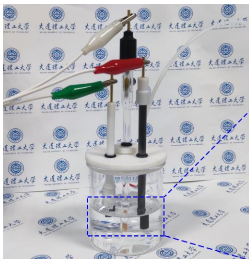
Figure S21. Digital photograph of a single-cell three-electrode setup.
