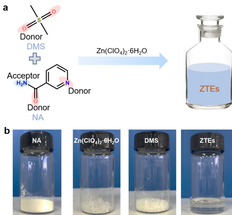
Figure S1. (a) Scheme for preparing the ZTEs. (b) Optical photographs of prepared ZTEs in a predetermined Zn(ClO 4 ) 2 ·6H 2 O/DMS/NA with molar ratio of 1:3:0.5.
