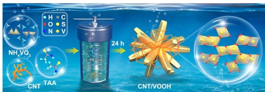
Figure S1. Schematic illustration of the synthesis of the CNT/VOOH composite.
