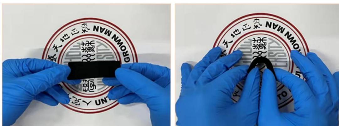
**Figure S5.** Photographs illustrating the flexibility of NiNF-1100.
