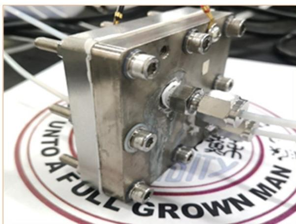
**Figure S26.** Photograph of a typical MEA electrolyzer with an effective electrode area of  $5 \text{ cm}^2$ .
