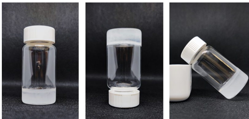
Fig. S3 Digital images of DOL/DME (v:v=1:1, with 1 M LiTFSI) after in situ polymerization (6 hours).
