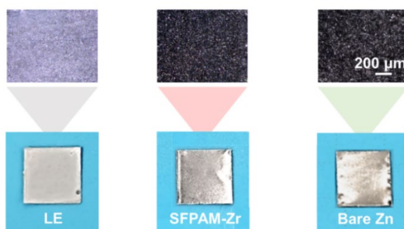
Fig. S11 Optical images of the Zn metal surface before and after covering with SFPAM-Zr and immersing in LE for 9 h.
