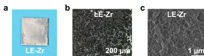
Fig. S12 The (a, b) optical and (c) SEM images of the Zn metal surface after immersing in LE-Zr electrolyte for 12 h.
