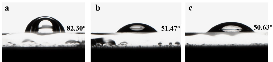
Fig. S11 Water contact angle images of (a) PTAA, (b) PTAA/DMF, and (c) PTAA/QA films.
