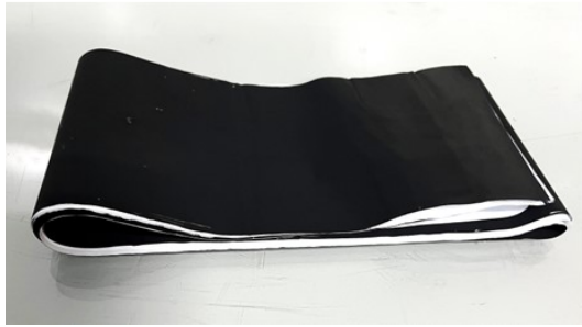
Figure S10. The stability of different separators under bending and wrinkling.
