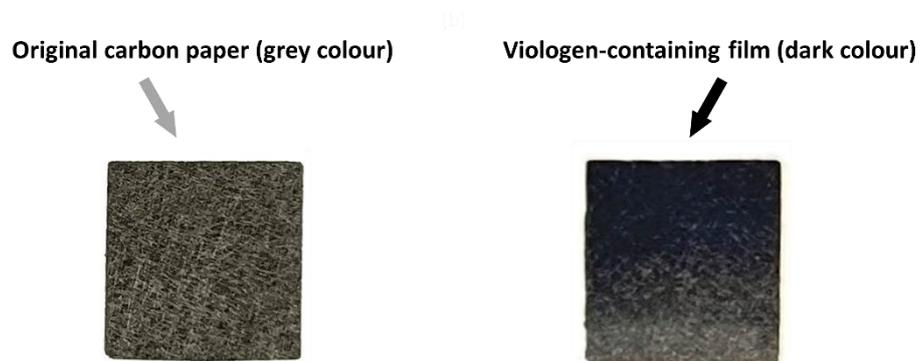
**Figure S2.** Illustration the formation of a viologen-containing film on the carbon electrode in the H-cell configuration, using 0.02 M BV in 1 M NaCl aqueous electrolyte: The original carbon electrode (left), viologen-containing film becomes visible after electrochemical reduction (dark colour, right).
