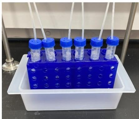
**Figure S1.** Illustration of the Lab-scale air contactor array setup, bubbling air into CVE-regenerated capture solution.
