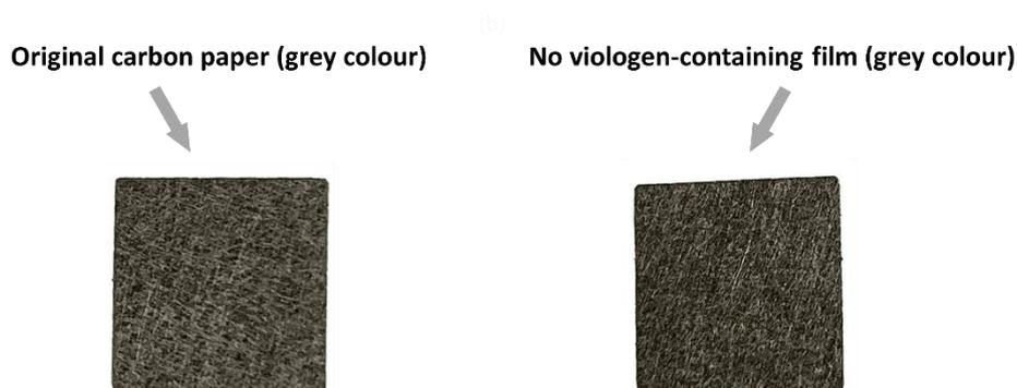
**Figure S13.** Illustration the carbon electrode in the H-cell configuration, using 0.02 M BPPV in 1 M NaCl aqueous electrolyte: The original carbon electrode (left), No viologen-containing film after electrochemical reduction (right).
