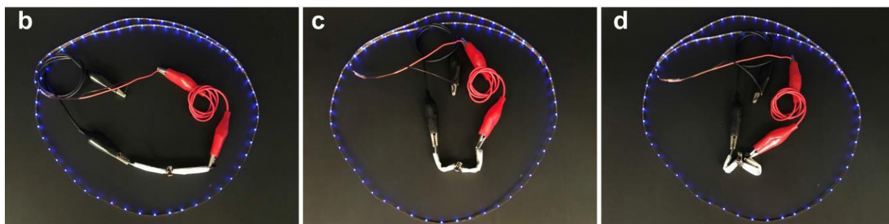
Figure S42. (a) Galvanostatic charge and discharge profiles for quasi-solid-state Zn-air battery containing \text{NiMoO}_4\text{-Fe-5}^{\text{th}} at 2 \text{ mA cm}^{-2} and different bending angles; (b) Photograph of a flexible Zn-air battery powering LED lights.
