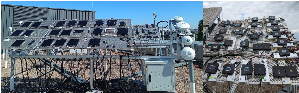
Figure S4 Outdoor test field in Berlin (Germany) comprising of the fixed tilted rack for solar cells, meteo station, MPP tracking equipment, spectrometers for measurements of the sun spectrum and additional irradiance sensors in the plane of array and temperature sensors on the rear of the cells. The photograph on the right shows research PSCs with area of \leq 1 \text{ cm}^2 which are investigated in this paper.
