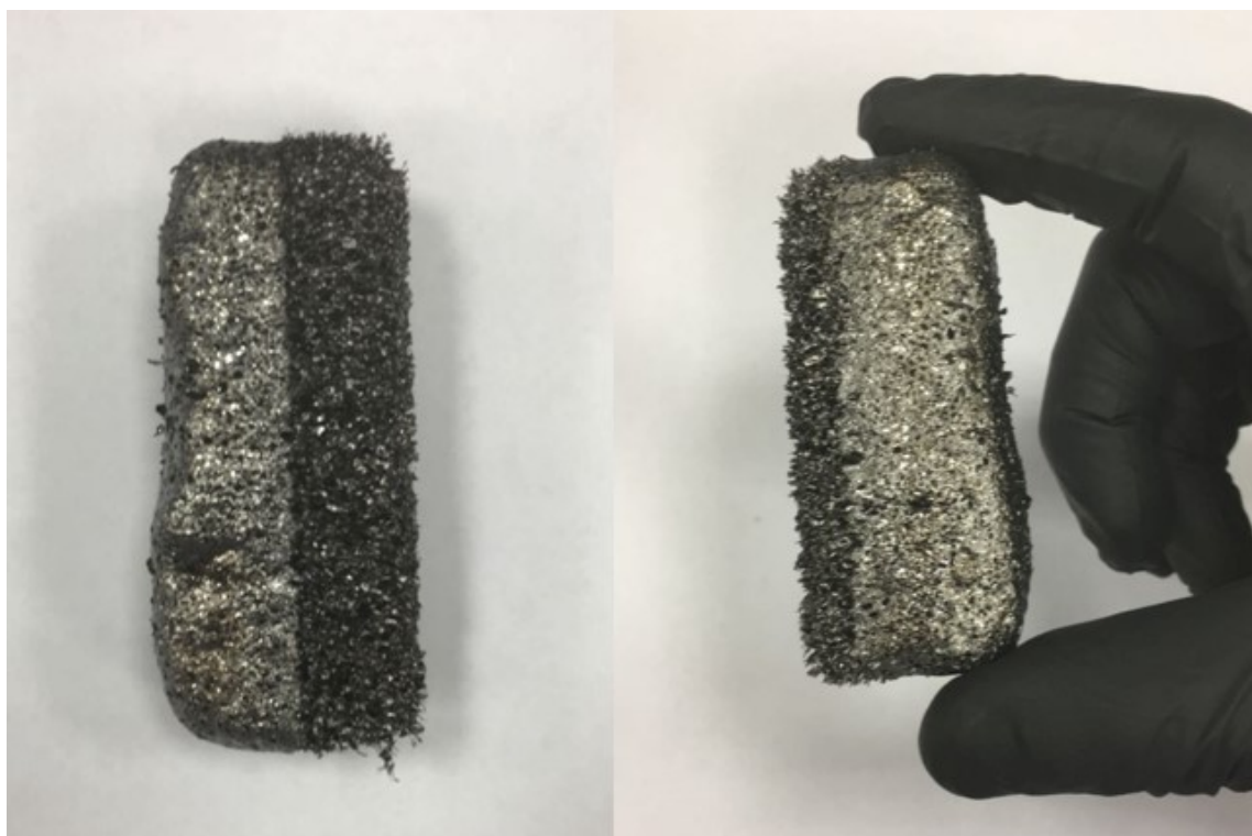
Supplementary Fig. 2 Photograph of the IL after carbonisation at 800 °C.
