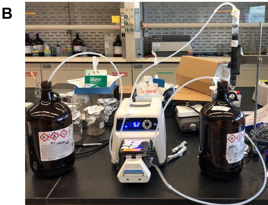
Figure S1. The flow-through leaching system setup. (A) Schematic diagram of the setup; and (B) photo of the leaching system setup in the lab.
