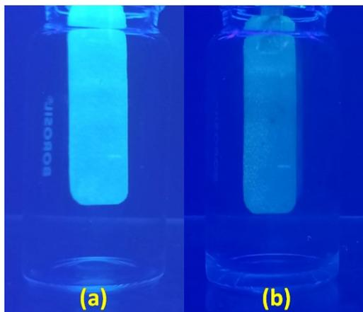
**Fig. S12** Filter paper strips loaded with ANO (1 mM) exposed to UV lamp (365 nm) to visualize fluorescence changes after 1 min (a) ANO alone (b) ANO + phosgene gas (50 ppm)
