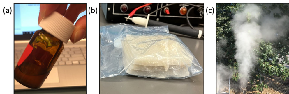
Figure S2. (a) Sample vial containing styrene-based resin, (b) pieces of cured composite that was powdered and suspended in ethanol, and (c) steam-laden waste released during CIPP installation that was condensed in cold traps at field sites.
