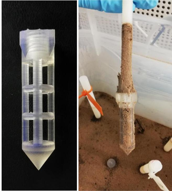
**Figure S6:** Sample holder without mesh bag (left, length = 5 cm, diameter = 1 cm) and during the sampling after the oxic sampling in redox cycle I at 4 weeks (right).
