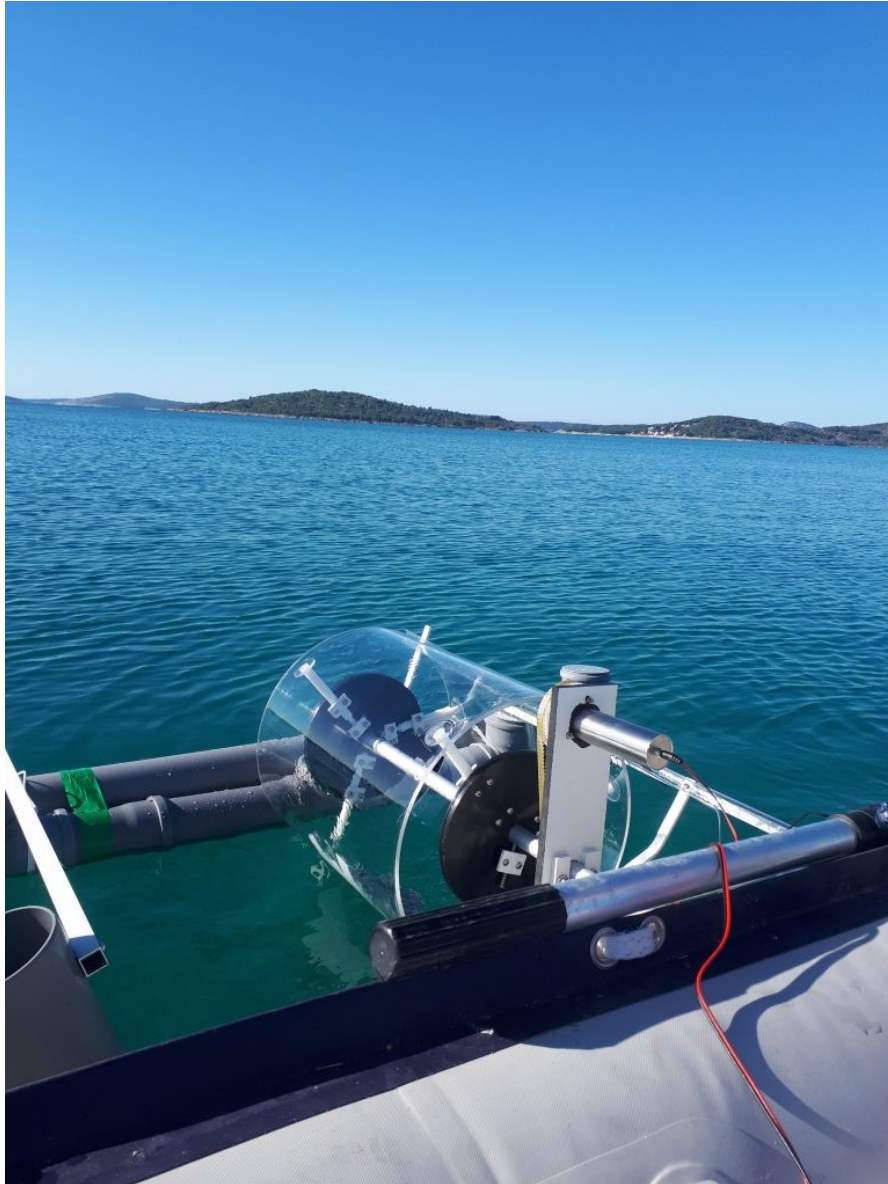
Fig. S2. The sea surface microlayer sampler (designed by dr. D. Omanović, Ruđer Bošković Institute, Zagreb, Croatia)
