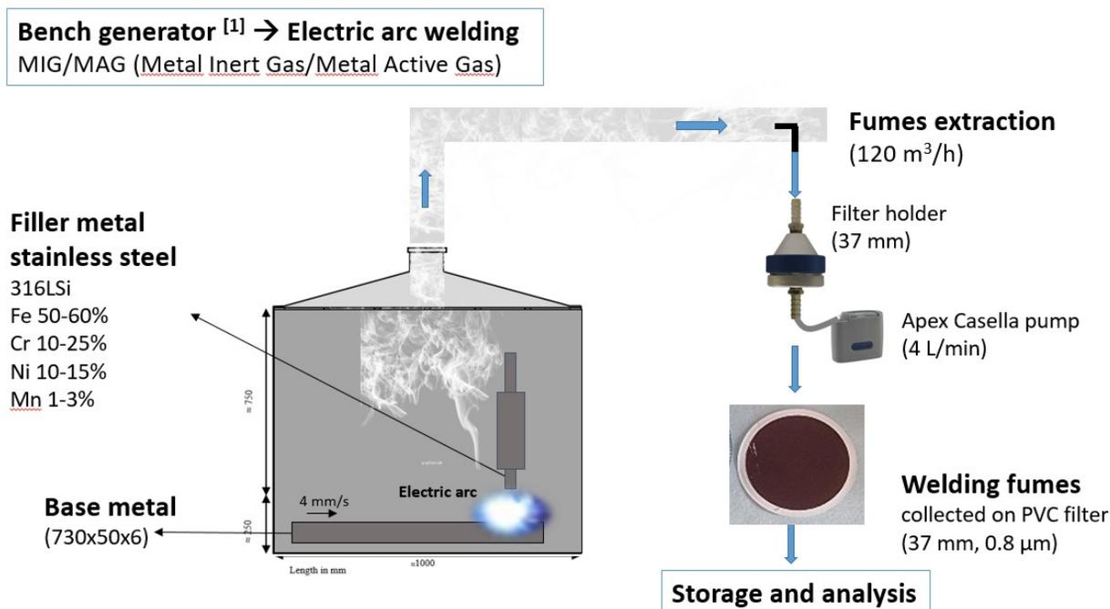
Figure S1. Welding fume generation bench<sup>1</sup>.
