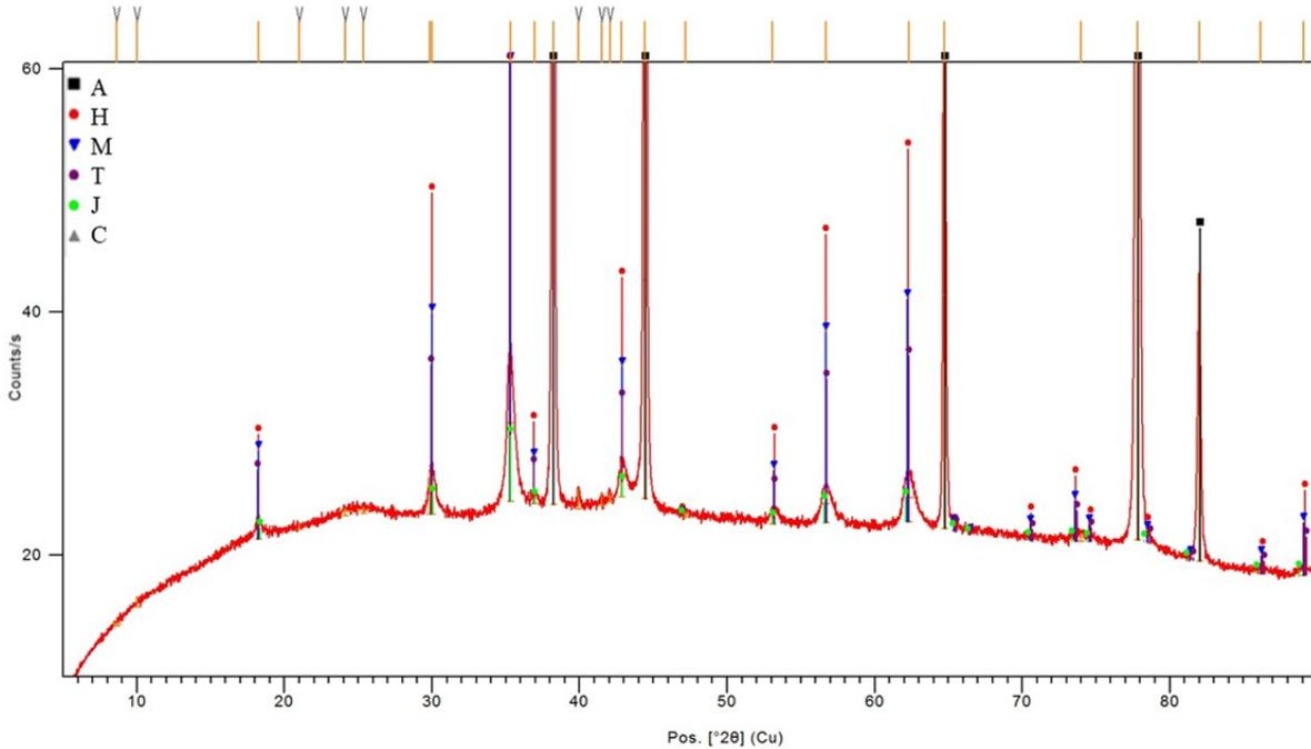
Figure S4. XRD spectrum of fresh WF generated on the welding bench. A : aluminum\*, H : magnetite Fe<sub>3</sub>O<sub>4</sub>, M : Manganochromite Cr<sub>2</sub>MnO<sub>4</sub>, T : Trevorite Fe<sub>2</sub>NiO<sub>4</sub>, J : Jacobsite MnFe<sub>2</sub>O<sub>4</sub>, C : Chromite Fe<sub>1.7</sub>Cr<sub>1.3</sub>O<sub>4</sub>
