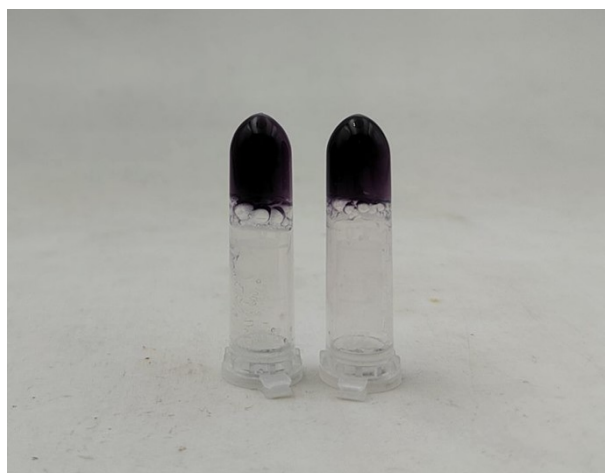
Figure S4. The nanoparticles appeared in reaction hydrogels at room temperature for 20 days without presence of \text{OH}^- .
