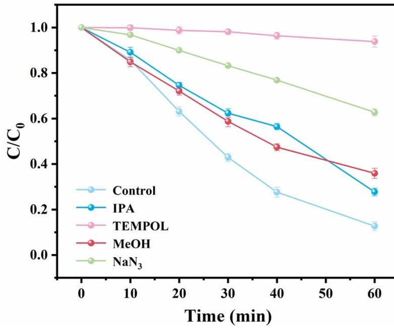
Fig. S4. Photocatalytic activity of 0.3BQBVO photocatalytic for NPX degradation under visible light with the addition of different scavengers.
