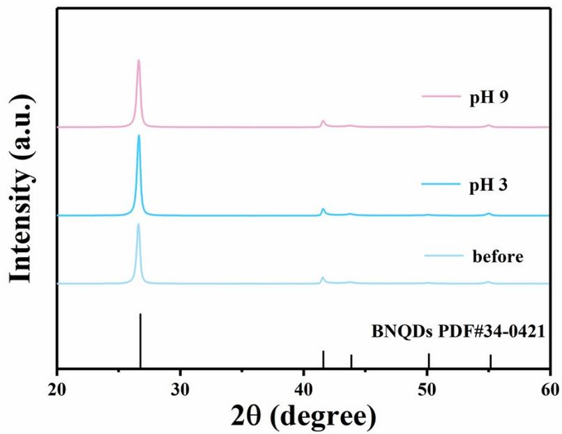
Fig. S6. XRD patterns of BNQDs, prior to and following photocatalytic experiments conducting in aqueous solutions with pH of 3 and 9.
