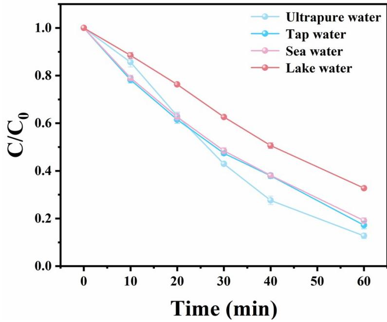
Fig. S5. Photoactivity under diverse aqueous matrices. (NPX:10 mg/L; Powder dosage: 500 mg/L).
