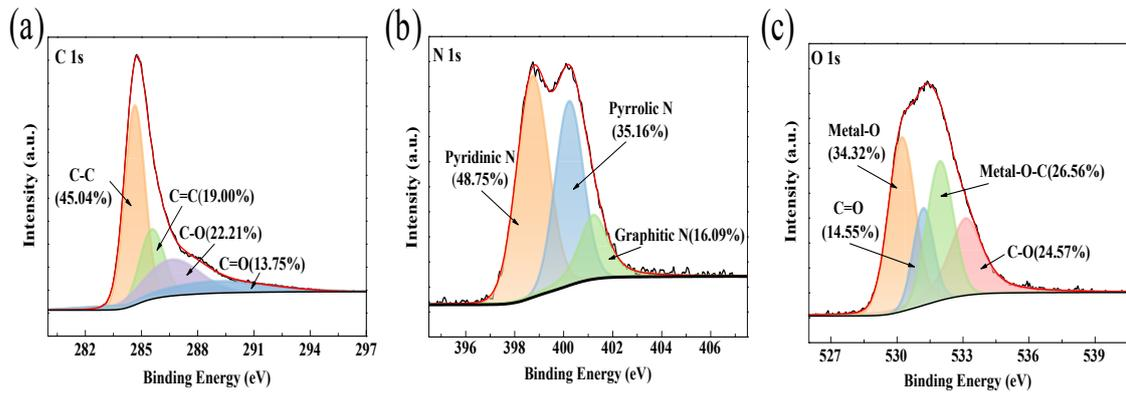
**Fig. S13. (a) C 1s, (b) N 1s and (c) O 1s spectrum of XPS of  $C_{1Ds}@CFO@F^0C^0$  after six times inactivation**
