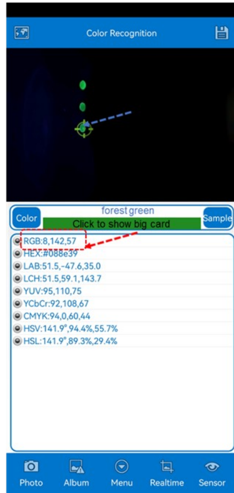
Figure S7 The RGB values recognized by smartphone APP (A and B) (the photograph was taken under 254 nm UV lamp).
