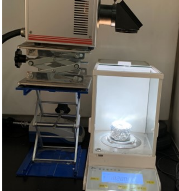
Figure S9 The photographs of home-built set-up for steam generation with the solar simulator.
