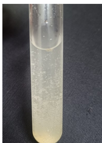
Fig. S12 Confirmation test for the presence of carboxylic acid functional groups on CNGdAg-40 % surface.
