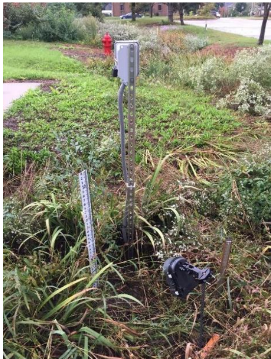
Fig. A1. The sensor validation setup using a gage plate and camera. 1
