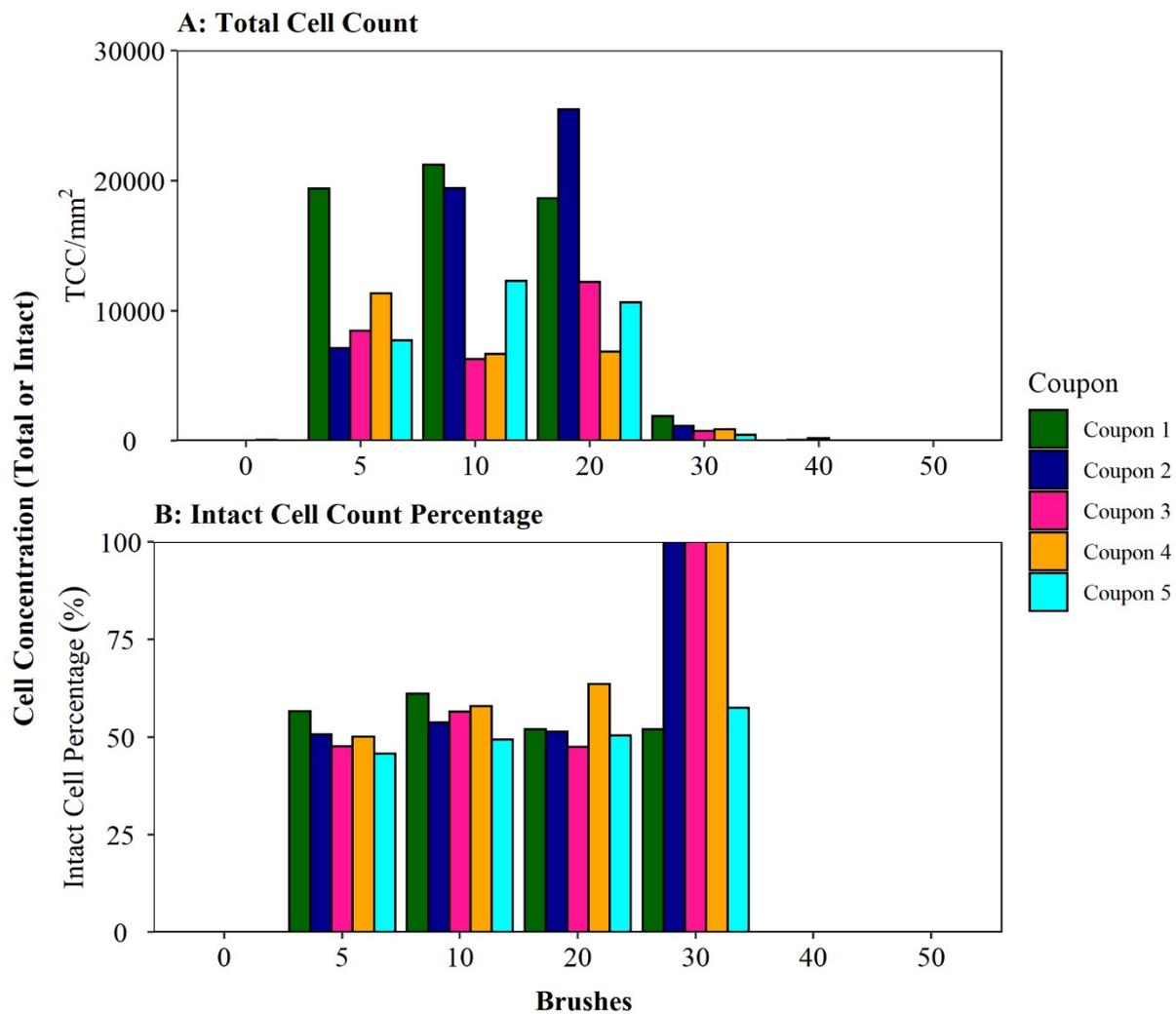
**Figure S5. Impact of brushing on cell viability when used to remove biofilm from coupons.** Coupons (n=5, see key) were brushed for a series of 0, 5, 10, 20, 30, 40 and 50 brushes. Total cell counts (TCC) and percentage of TCC that were intact are presented. 0 brushes is defined as phosphate buffer solution (PBS) poured over the surface of the coupon to act as a control.
