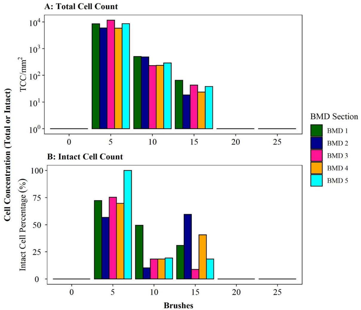
**Figure S4. Impact of brushing on cell viability when used to remove biofilm from a Biofilm Monitoring Device (BMD).** BMD pipe sections (n=5, see key) were brushed for a series of 0, 5, 10, 15, 20 and 25 brushes. Total cell counts (TCC) and percentage of TCC that were intact are presented for each replicate. “0” brushes is defined as phosphate buffer solution (PBS) poured over the surface of the coupon to act as a control.
