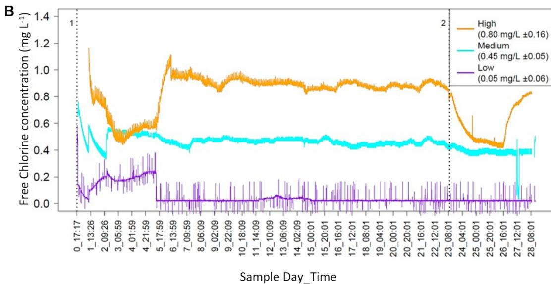
**Figure S2 Full-scale pipe loop facility (A) and residual chlorine concentrations (B) during biofilm growth.** A. Three independent high-density polyethylene (HDPE) pipes, 203 m long with Pennine Water Group Coupons facilitating biofilm sampling. B: residual free chlorine concentration, raw data is plotted ( $n \geq 39986$ ), average  $\pm$  standard deviation. 1 = dosing started, 2 = dosing interrupted in High-chlorine for ~48 hours. Adapted from Fish et al., 2020.
